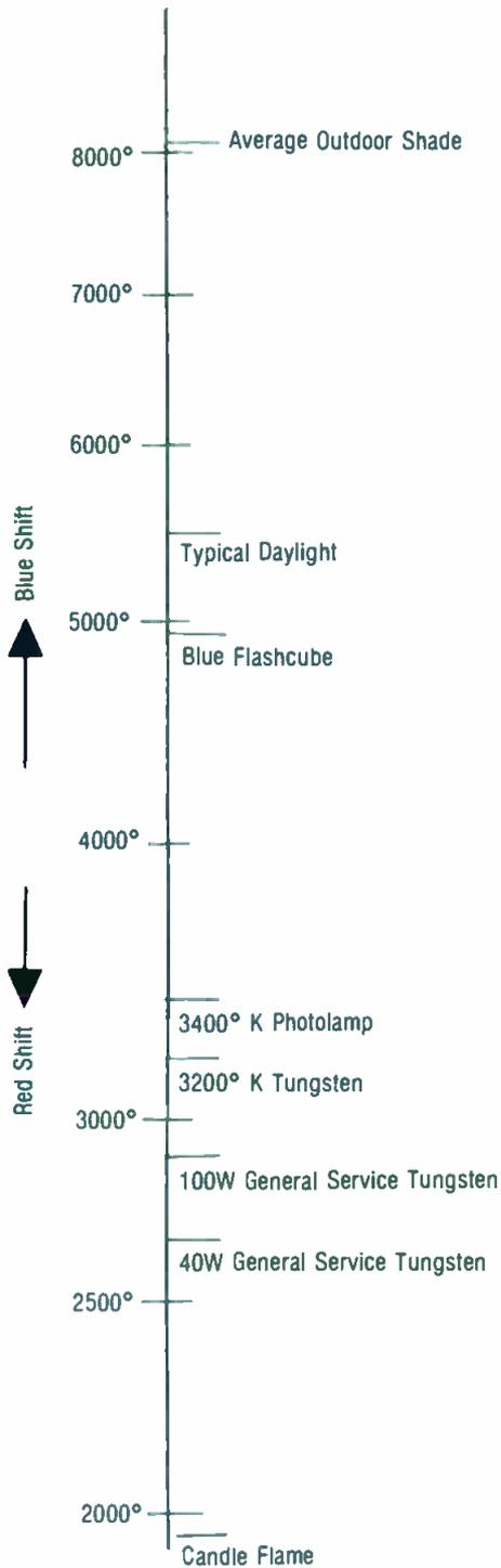
Figure 9. Kelvin temperature of typical light sources.
