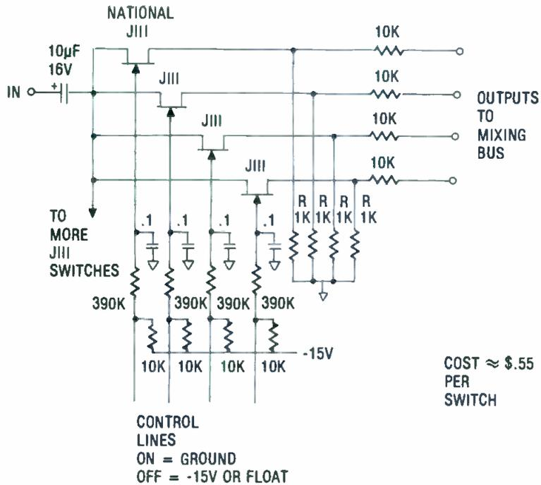
Figure 3. JFET switch building block.
