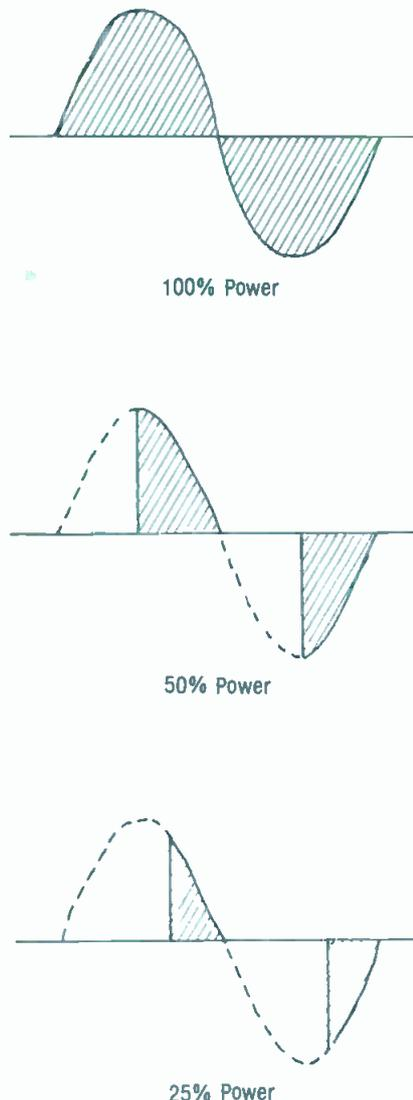
Figure 11. SCR dimmer output waveforms.
