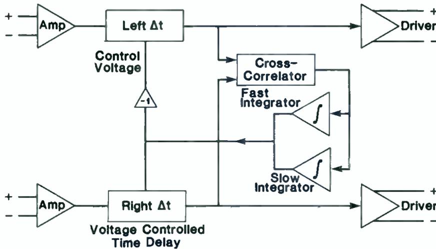
**Figure 2.** Block diagram of the active phase corrector. Output signals are time-aligned, thus eliminating a stereo phase error. A detector performs a time-phase analysis on regular program material to sense a phase error. Feedback loops to analog display lines correct the error.
