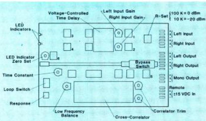
**Figure 6.** Phase chaser electronic layout.
