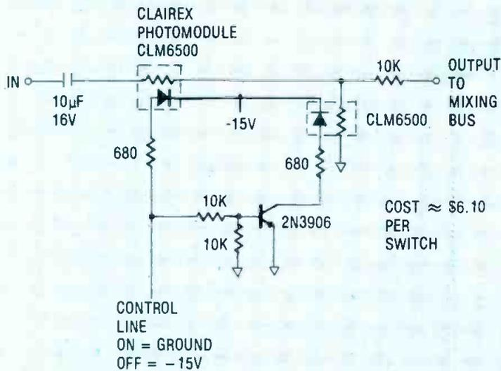
Figure 4. Photomodule SPST switch building block.
