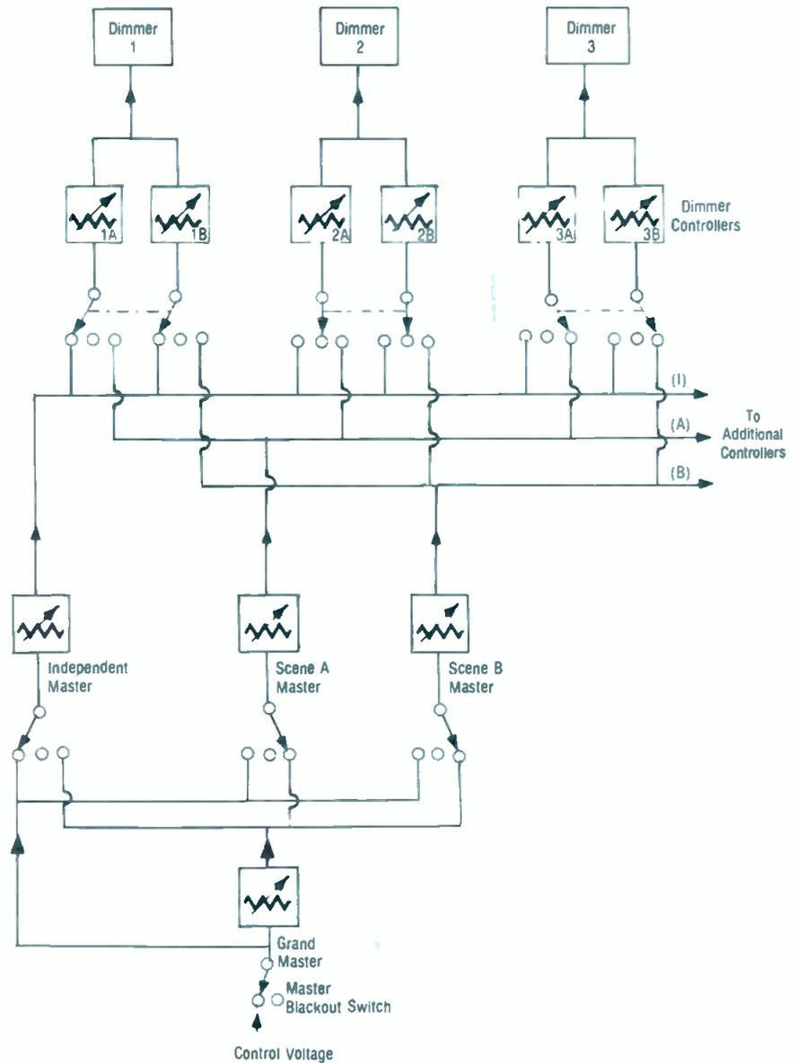
Figure 17. 2-scene preset control with independent master and grand master.
