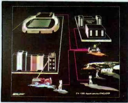
Fiber-optic cables weighing five pounds per 1000 feet connect the minicamera to the van over distances up to two miles, in locations where portable microwave cannot be used.
