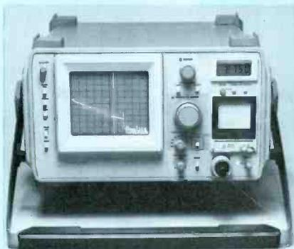
vides quantitative and calibrated measurements of high accuracy and reliability. Precision-calibrated loss and distance measurements are possible with this rugged, portable instrument. A chart recorder for documentation complements the CRT display for measurements on multimode 125µm OD fibers with a core diameter of 50µm.
