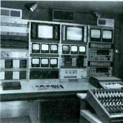
The vehicle is built around an all-aluminum step-van body. It features four Ikegami ITC-350 color camera capability, an Electro-Voice audio console, a Crosspoint-Latch 6112 special effects switcher, dual Sony VO-5850
