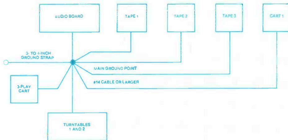
Figure 2. Ground system layout for individual equipment rooms.
