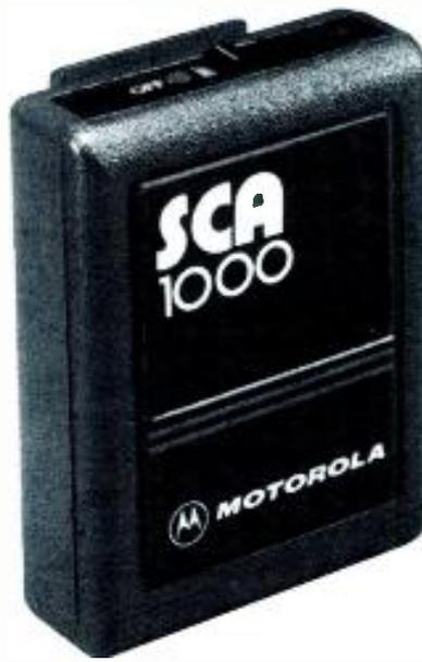
The Motorola SCA-1000 Tone Alert radio pager can be set to receive SCA transmissions from any one channel in the FM broadcast band.
