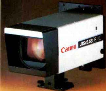
**J15x8.5BIE** for 2/3" cameras. 2/3" Economy—full utility for all studio situations, combining a 15X zoom ratio with an M.O.D. of under two feet, a 54° angle of view and high sensitivity throughout the range.
