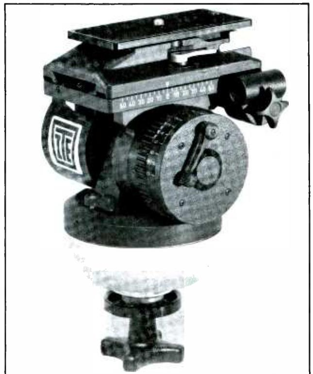
Innovative Television Equipment has announced the ITE-H70 heavy-duty fluid action head, designed to support (with Mitchell base adapter) camera loads to 65 pounds. Weighing 19 pounds, the fluid head is equipped with a 150mm claw-ball base, adjustable quick-release camera plate, spirit level and dual-control handles. The fluid head interfaces
