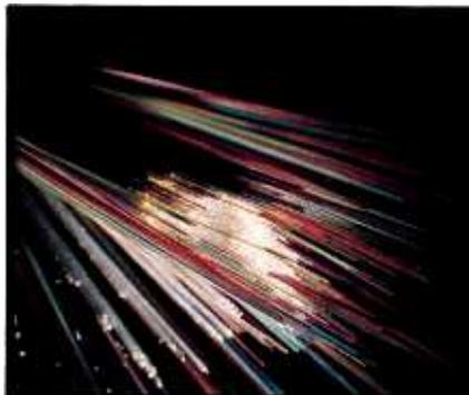
transfer of information by photons (light) through an enclosed medium such as glass or plastic fiber. The fundamental process is somewhat analogous to electrons passing through a metallic conductor such as wire. However, the analogy ends there. The components most common to a fiber-optic system are the transmitter, which converts electrical energy to light energy; the fiber, which is the conduit of that energy; and the receiver, which converts the light energy back to electrical energy.
