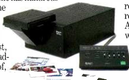
System includes Video Image Recorder, control console, and print film camera/adaptor. 35mm camera/adaptor optional.
