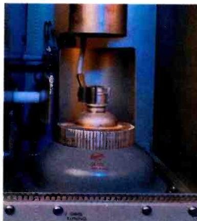
EIMAC's 5CX1500B broadcasting tube in KGLT radio station's transmitter.
