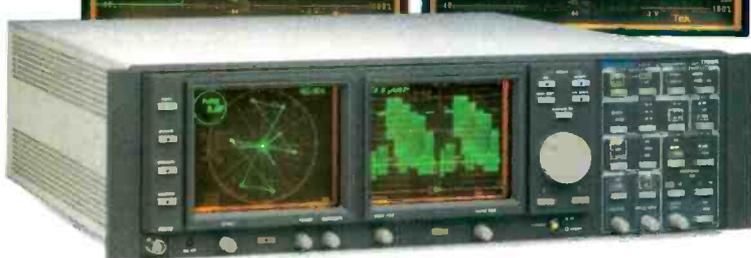
Even at first glance, you can see that the Tek 1780R is in a class by itself. Only the 1780R offers full-bandwidth analog measurement capabilities with separate, complementary waveform and vector displays. Component and composite capabilities are provided through four video inputs and a front-panel probe
