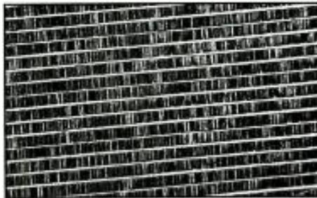
The trend toward increased recording density is clearly visible in these magnetically “developed” micrographs. At left, a 50× magnification of Betacam’s component analog format is shown (darker tracks are C, lighter tracks are Y). At right, the component digital D-I format is shown at the same magnification. (Courtesy of 3M.)
