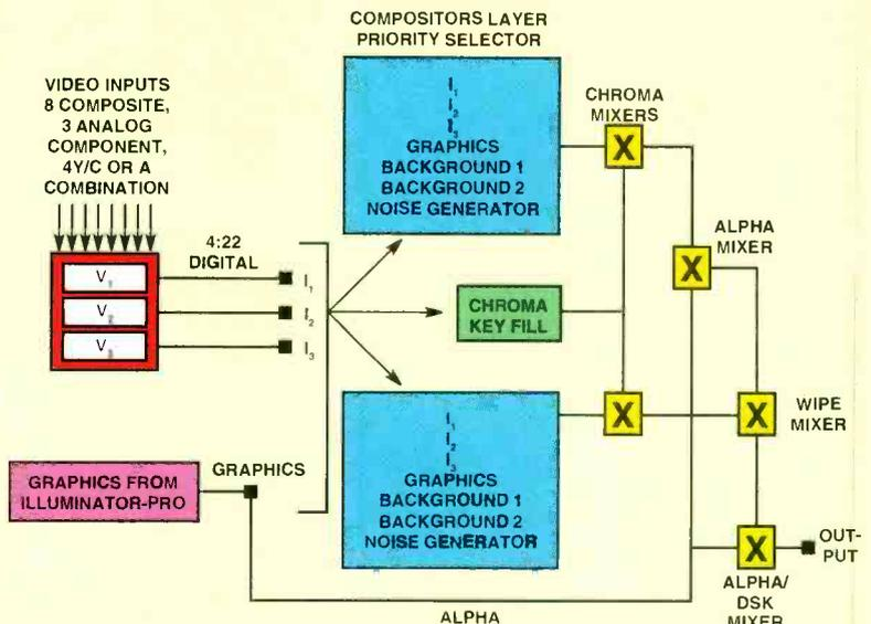
Figure 1. A block diagram of the Matrox SIESTA device.
