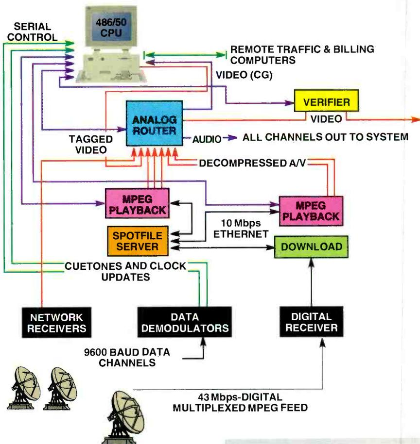
**Figure 1.** Digital satellite delivery of commercials can tie even the most remote cable systems together as an interconnect, or transport national and promotional spots for near immediate turnaround.
