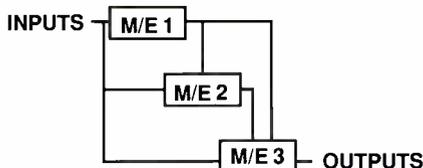
Figure 1. The concept of a mix/effects switcher.
