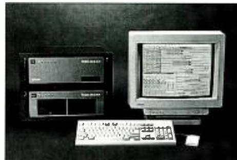
• **Timeline Studioframe edit controller:** offers users a high-resolution scrub/jog wheel for precise machine control and editing functions, as well as dedicated track access keys to all tracks; features a set of software-configurable control keys that can be mapped to a floating toolbar in the application menu; user can assign menu functions to the keys, making software functions hardware ones.
