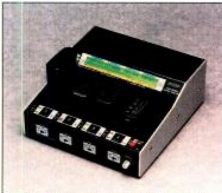
• **Cadex C4000:** services NiCd, NiMH and SLA batteries; more than 700 battery adapters available for portable radios, cellular phones, laptops and cameras; battery parameters stored in adapters, eliminating the need to set the analyzer to a specific battery; optional printer interface.
