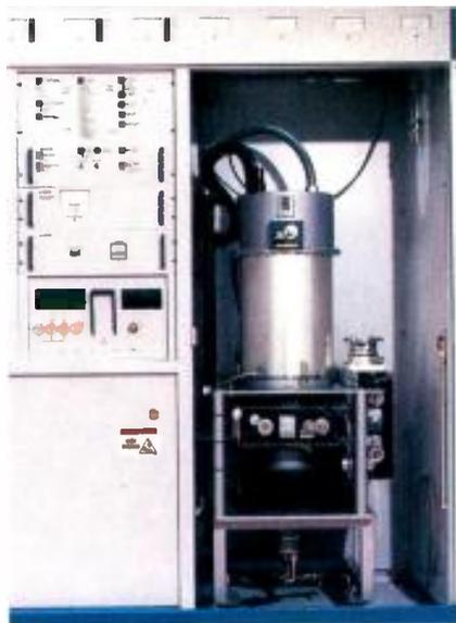
IOTs are presently available for 40kW and 60kW visual service and combined amplification powers of up to 42/4.2kW.
