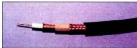
• **Model LVT61859S:** 75Ω triax video cable for use in remote applications; 21 AWG (19x34 AWG) stranded copper center conductor; insulation constructed of high-density cellular foam polyethylene for crush resistance and low capacitance; two shields are constructed of 95% coverage-braided copper; all-weather jacket enhances the cable's flexibility; currently available as a stock item.
