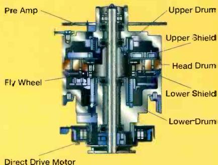
To ensure S-VHS compatibility, the drum structure features an upper stationary drum, a middle rotary drum, and a lower stationary drum. To eliminate the need for a thicker air film at the drum inlet and to provide stable head-to-tape contact, the thickness of the rotary drum is very narrow. The end result of this configuration is the truest track linearity. The inner drum's tapered shape also reduces tape damage, powder drop, wear and burn.
