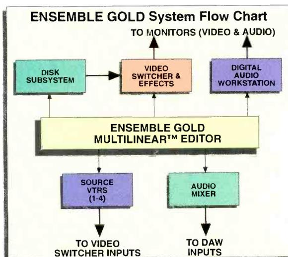
Figure 1. Basic system layout of a typical Ensemble Gold system.
