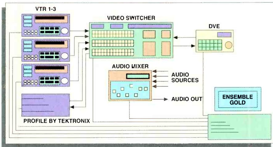
Figure 3. By incorporating the Ensemble Gold, this linear system has been expanded to include non-linear along with linear in one complete package. This system is using all external devices for DVE switching and audio, while the Tektronix Profile is providing digital betacam quality.
