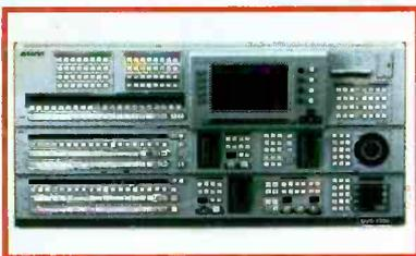
variety of visual effects and operational flexibility; like the DVS-7000, it can be used at component or composite stations; the DVS-7200 features two mix/effects banks, each with two full-function keys.
