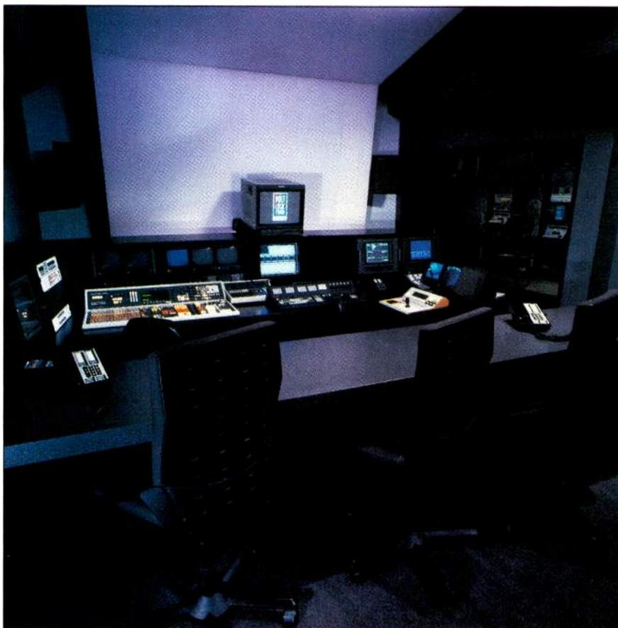
Traditional edit bays such as this one located at Post Logic Studios, Hollywood, operate in the uncompressed domain of SMPTE-259M. However, as we move toward DTV, facilities such as these may also have to handle compressed signals.
