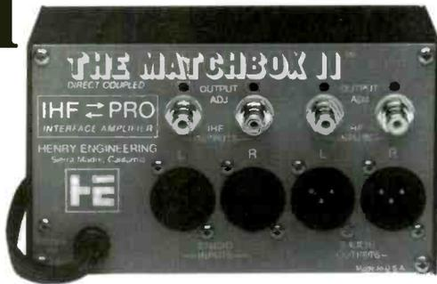
Get Matchbox II to convert "consumer" (RCA and mini-jack) audio inputs and outputs to "600 ohm" balanced lines at +4dbm professional levels. Eliminate the hum, buzz, and distortion caused by mismatched levels and impedances! Gold plated connectors and direct-coupled, active circuitry yield superb audio performance. Over 20,000 units in use worldwide!
