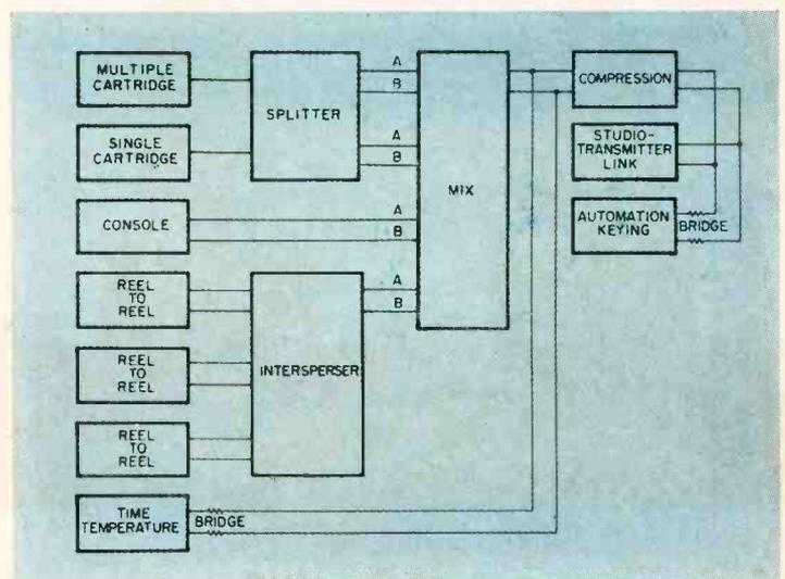
Block diagram of the WKLS automated programming equipment setup.
