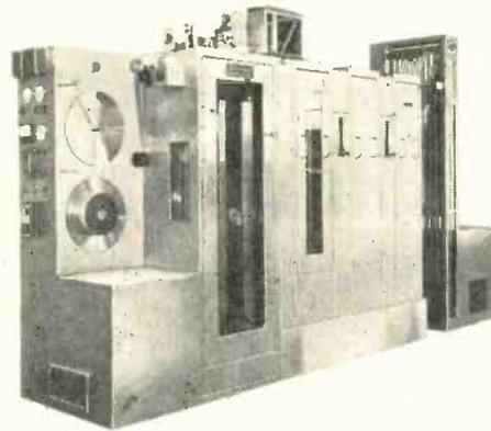
They work continuously, without downtime, maintenance problems or lost film. Unmatched reliability and quality have been characteristic of all Filmline processors since 1947.
