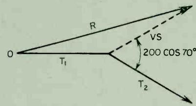
Fig. 8. The effect of space phasing on the vectorial relationship.
