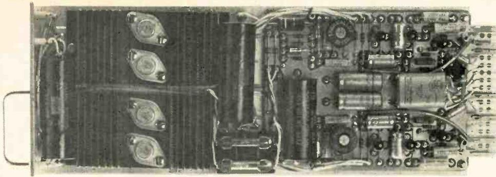
AA-601 Plug-in Audio Distribution Amplifier Module (with cover removed) — self contained, solid state design. Each module provides up to 6 outputs (60 in a 5 1/4" frame) at +24 dbm, 600 ohms balanced.
