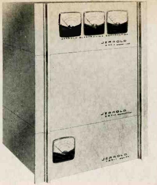
The heart of an ETV system is the radio link between the studio and each individual school building. The Jerrald SRT-1 transmitter is designed for multiple channel output mixing, and the exciter-modulator and control unit (one required for each channel) can be mounted any distance from the transmitter. The mast-mounted receiver will pick up any 4 or 5 alternately-spaced VHF channels.
