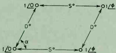
Fig. 5. Typical parallelogram or rhomboid tower configuration.
