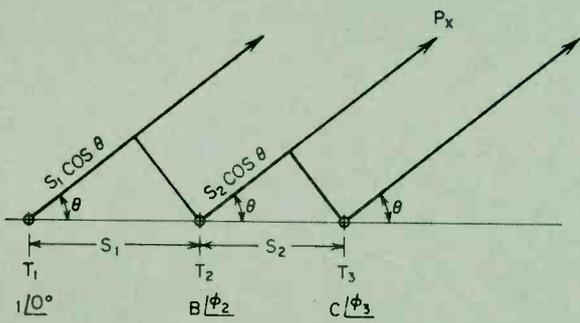
Fig. 2. Vector relationship of simple 3-tower array.
