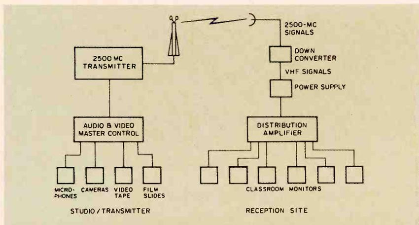
A typical 2500-mc ETV system beams program material originating from live studio, video tape or film machine to each building equipped with a receiver. 2500-mc signals are converted to VHF channels and distributed by cable to each classroom outlet.
