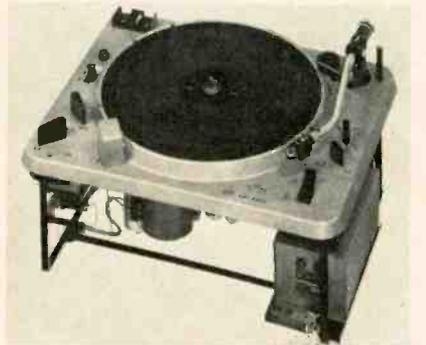
The turntable is equipped with remote start/stop control and is said to reach operating speed in 0.4 sec., with output cutoff for wowless starts and cueing to the beat or syllable. Incorporates synchronous motor, arm lowering device, groove illumination light, and interchangeable mono and standard groove cartridges. Price, less console, is \$1295.
