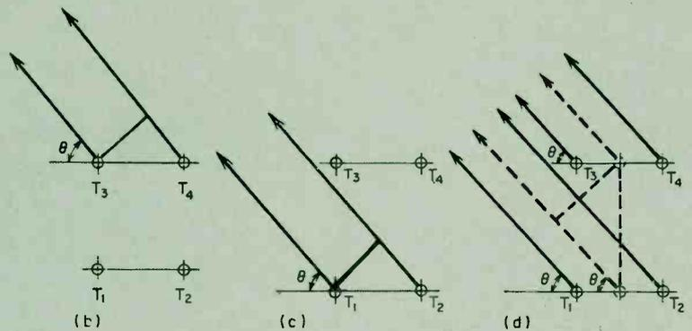
Fig. 4. (a) 4-tower array with symmetrical pairs; (b and c) vectorial treatment of each pair of antennas,  $T_1$  and  $T_2$ ,  $T_3$  and  $T_4$ ; (d) vectorial combination of the 2-tower pairs.
