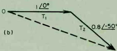
Fig. 7. Typical vectorial representation of a 2-tower array.
