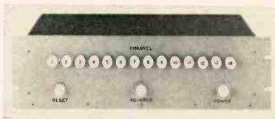
switching of 14 twinaxial input channels to a single twinaxial output. Switching is controlled by either front panel push button or remote contact closure. A reset or homing function is also provided with both front panel and remote
