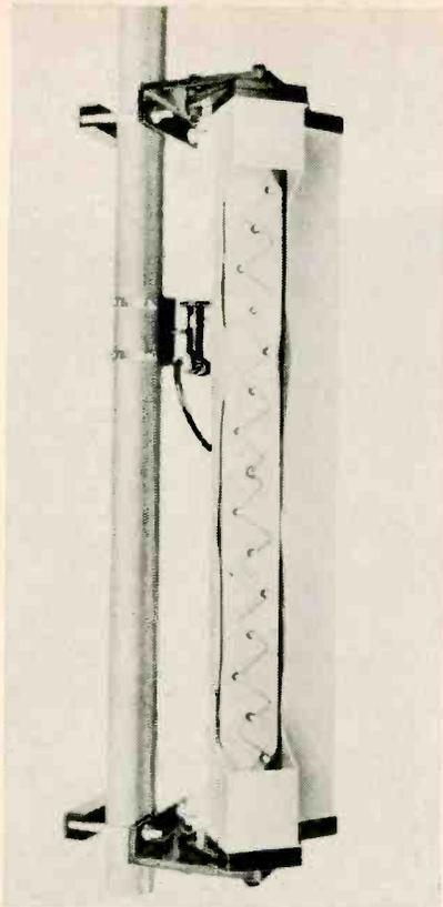
Example of newly developed zig-zag transmitting antenna developed for tailoring 2.5-kmc coverage pattern (Courtesy TACO).
