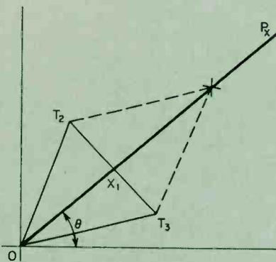
Fig. 3. Vectorial representation of 3-tower symmetrical array.
