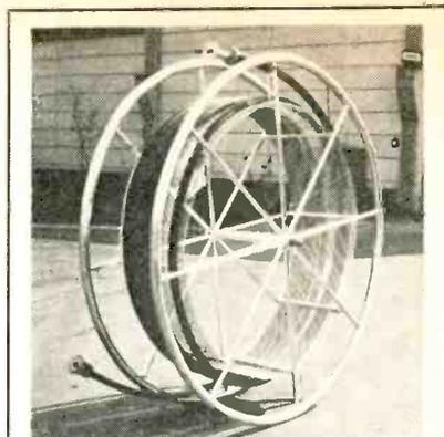
Heliac flexible waveguide for use in emergency restoration of 6- and 11-gc microwave systems available from Andrew Corp. Types EW56 and EW107 are being packaged on portable aluminum reels in various predetermined lengths with end fittings attached. In the event of failure, a transmission line section can be replaced quickly.
