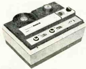
ips. The Wollensak VTR-150 uses a 1-inch diameter ferrite helical scan recording head; runup time is 8 sec. with two-motor drive. Specifications include: 2-mc bandwidth; signal-to-noise ratios: video; 35 db, audio, 40 db; wow and flutter 0.3%; audio frequency response from 50 to 100,000 cps  $\pm 3$  db. Tentative price is \$1495. Also will be available in mobile console package at less than \$3000, including camera, tape, monitor receiver, mic headset and accessory cords.
