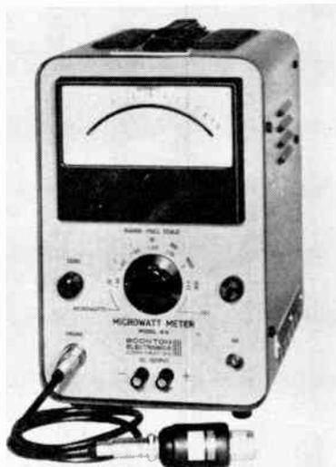
quency range of 0.1 MHz to 6 GHz and has maximum sensitivity of 0.001 microwatt per hour; no zero balancing is required on any but most sensitive range. VSWR is less than 1.2 up to 2.5 GHz and less than 1.5 to 6 GHz; accuracy is said to be ±0.5 db. Meter scale is calibrated in microwatts and dbm. Power detector is equipped with type N connector for 50-ohm system Price is \$695.
