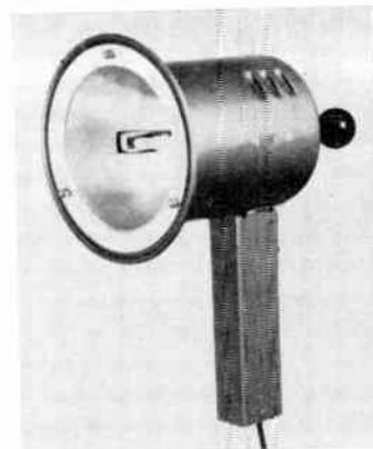
3 provides full focusing from spot to flood and weighs 2 lbs. 10 oz., produces 220 ft. candles at 10' in spot focus and 56 ft. candles in flood focus. Model LQK-3 is a medium flood with fixed focus; weight is 1 lb. 12 oz. and it produces 160 ft. candles at 10'. 30v nickel-cadmium battery (Model PBC-30/2) with detachable charger will permit 30-min. operation from fully-charged battery.
