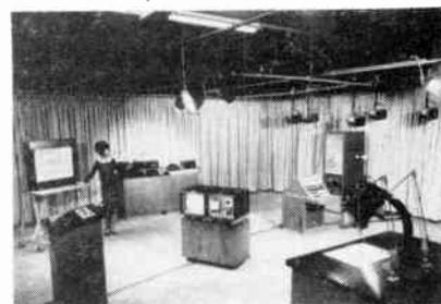
clock, background drape, tape punch, tape reader in rack cabinet, sync generator, distribution amplifier and video sync mixer. By punching camera sequence on paper tape in advance, the teacher can operate all equipment with a single hand-held control button and move around at will. An auxiliary console is available: options include a VTR, viewfinder camera, and EIA sync. Price is \$22,000.
