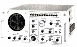
Measuring amplitude changes and phase shifts can be done accurately, conveniently, and independently with the Vectorscope. The Vectorscope presents relative phase and amplitude displays (of chrominance information in the N.T.S.C. color signal). Dual-trace capability permits simultaneous display of two color signals for precise matching of phase and amplitude. In addition to the vector display, the Vectorscope
