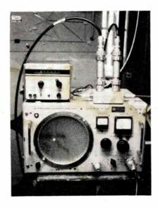
Figure and photo show test setup used to measure impedance and vswr at WNEW-TV. Photo shows spot of light projected on Smith chart showing measurements.
