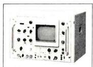
SWOF VIDEOSKOP provides dynamic plotting of envelope delay when used with Type LFM.
