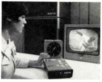
metal discs instead of magnetic tape, is capable of instantaneous replay of televised action at normal, fast and slow speeds down to frame-by-frame stop action. Its capabilities also include reverse action playback or analysis of highlights.
