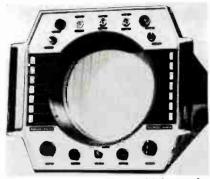
plan position indicator which can be installed up to 200 ft from the transmitter-receiver location. The peak power output of the transmitter, which operates on the 9345- to 9405-MHz band, is 20 kW. Pulse width is 0.6  $\mu$ s; pulse repetition frequency is 1000 Hz. I-f bandwidth is 5 MHz. When unit is operated on 115 or 230 V ac, power consumption is less than 500 W.
