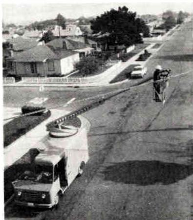
and is priced within the range of power ladder trucks. 125-in.-wheelbase model has basket that reaches a working height of 34 ft, and a
