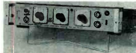
variable over  $\pm 500$  kHz. A precision attenuator and fixed pad permit continuously variable output power of 0.3 mV to 0.3 V (rf) and 1 mV to 1 V (i-f). Frequency response is better than  $\pm 1$  dB. Distortion typically is less than 0.2 dB and spurious deviations are less than 15 Hz. Price is \$995.
