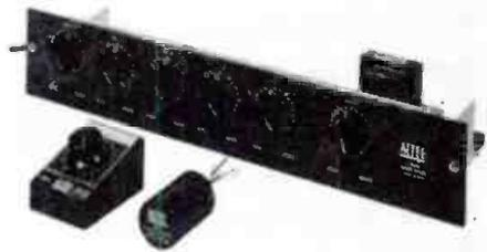
ing to remote unit location. The 1521A slave network, the heart of the Revocon II, will not change any of the performance characteristics of the original amplifiers. Up to six 1522A remote volume control units may be ganged from a single 1583A power supply, and the units may be bolted together to form a console of individual units for table or wall mounting, or portable operation.
