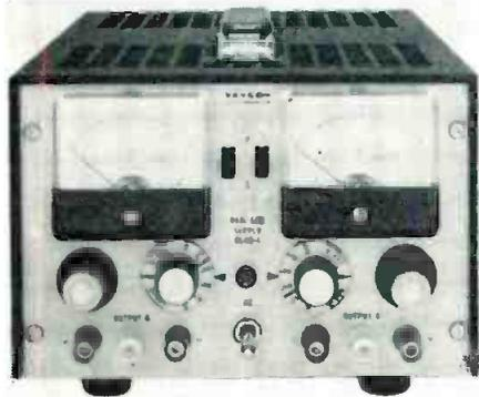
selection of 0.75 or 1 A for the 0-20 V range or 0.50, 0.1, 0.25, or 0.5 A for the 0-40 V range. Other features include input range of 100-125/200-250 V ac, 47-420 Hz. 0.01-percent regulation, 2 mV peak to peak ripple, and remote voltage programming and sensing. Price is \$249.
