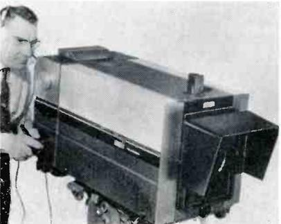
E.M.I. Electronics, Ltd., of London, processes signals from four lead oxide tubes, producing R, G and B for direct application to standard NTSC encoders and to standard RGB color monitors. Measuring 29 × 15 × 15 in. square, including zoom lens, camera uses direct imaging optical system
