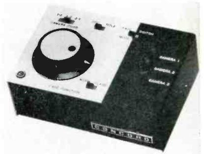
sure flare fade and superimpose images from a two- or three-camera system. TCP-1 may also be used with any multiple camera system employing an external sync generator. Provision is made for tally light, mic, or other desired connections between operator and cameras. Panel includes video inputs for up to three cameras and a video output for connection to videotape recorder. Panel measures 7 1/2 × 5 1/2 × 3 1/2, weighs 3 lb, and is priced at \$150.
