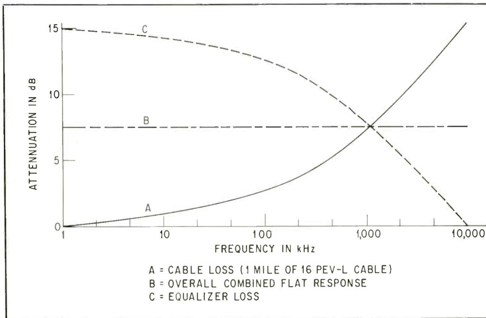
**Coaxial transmission lines used in telco loops don't have flat frequency response. Getting a flat output takes some fancy legerdemain to boost high frequencies at the sending end, which must then be attenuated at the output. The result is a better color program, but oh that test equipment setup!**
