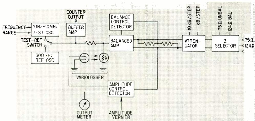
Fig. 4. Block diagram of the type 653A oscillator.
