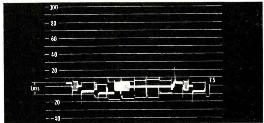
Using reference input of longest camera chain, time delay between signals will show on scope. Here, there's no delay.
