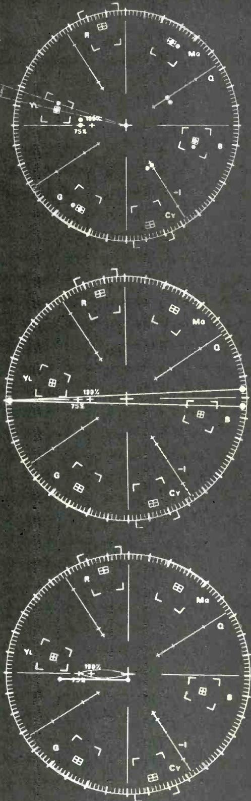
(Top) Vectorscope screen showing two signals when operating in the time-sharing mode. One of these signals is about  $4^\circ$  clockwise from the other. (Middle photo) By doubling vector amplitude and repositioning the display, physical displacement of signals will be doubled, increasing accuracy by factor of 2. (Bottom) Properly timed incoming system subcarrier displayed on the Vectorscope as a reference signal.
