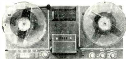
dynamic range and channel crosstalk are in excess of 30 dB. Continuous monitoring detects recording malfunctions, indicating which track is deficient. In case of failure, transfer of all operations to a standby recorder is automatic. All modes of operation are relay controlled from momentary contact pushbuttons. Any number of remote stations may operate CRM with complete indication of modes.
