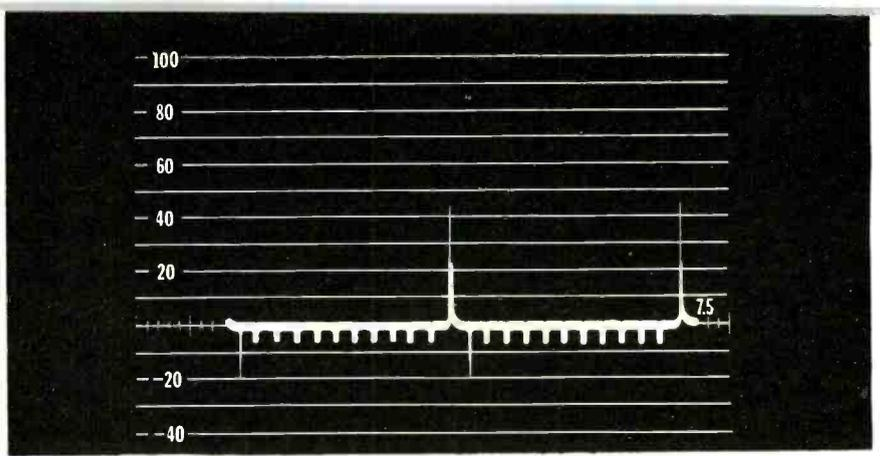
Spikes are due to time differences between two signals (path length through the system) and possible waveform modification.
