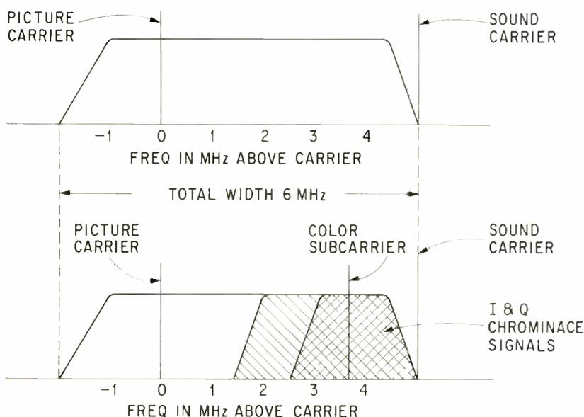
Fig. 2. Frequency spectrum of transmitted TV signals.
