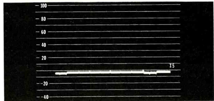
A time delay between the two compared signals shows up this way on the scope.
