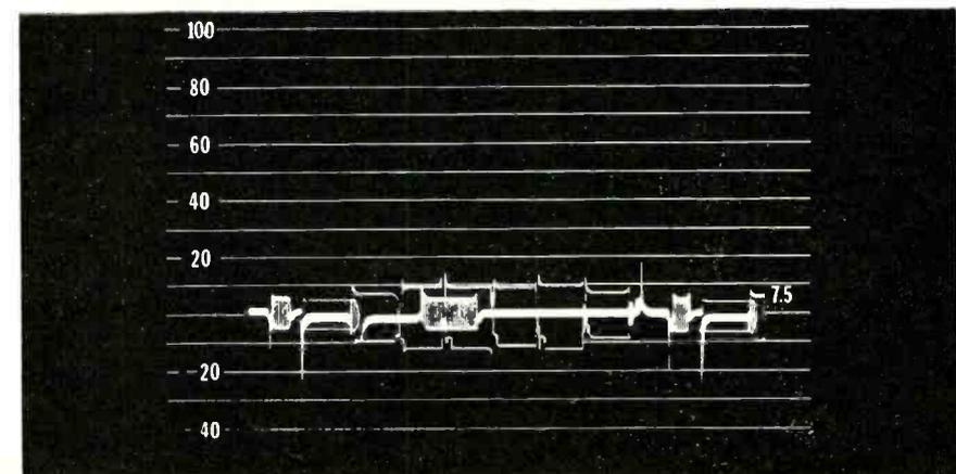
display on the waveform monitor, the trace is monitored for time delay between two signals as well. When both input signals arrive at the waveform monitor with no delay time difference between them, the waveform monitor will display a straight line when the vertical mode selector set for A-B.
