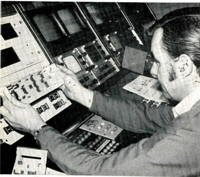
Changing pinboards in WXTV's master control takes only a few seconds, and can be done while an automated event is in progress.
