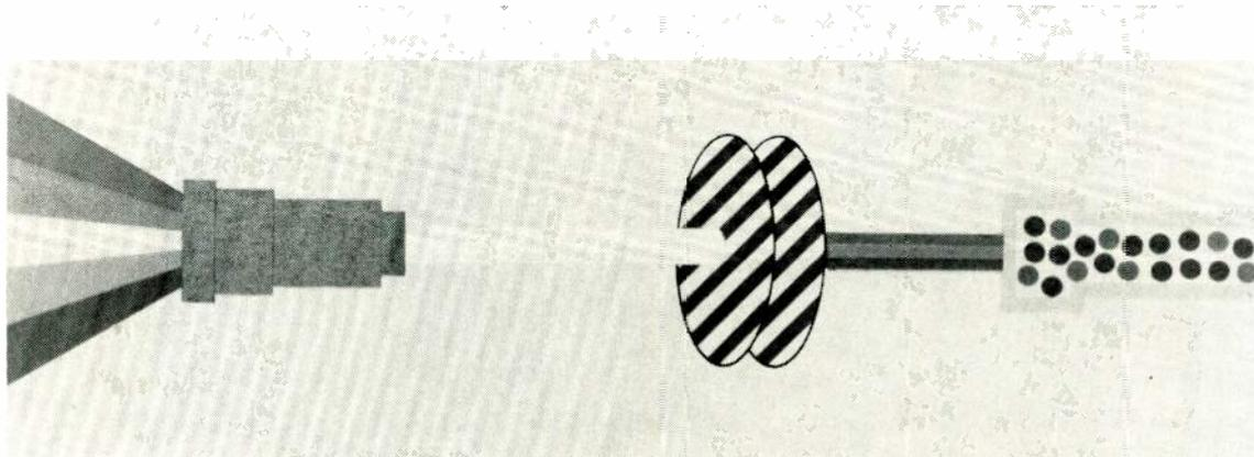
Light entering PK-730 lens (at left) passed through two overlapping filter grids to separate color information.
