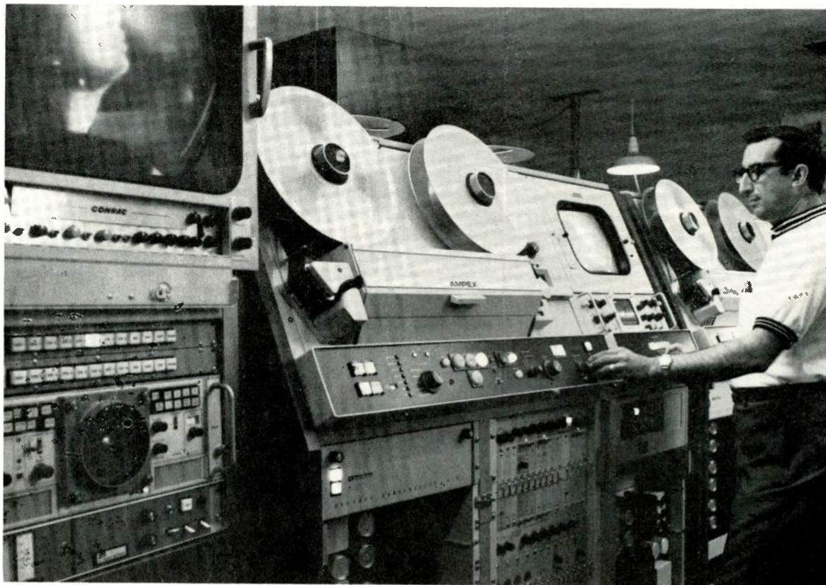
Four Ampex VR-2000 video tape recorders at KCET, Los Angeles, are used for delayed playback of west coast NET shows.
