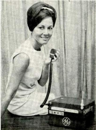
quarters, but are also recommended for portable and vehicle-installation use. The equipment, which has ac power as well as battery packs, may be used in 25-30, 132-174, 406-420 or 450-470 MHz systems. Base stations include noise-canceling mikes, handsets, two-frequency transmit and receive, solid-state channel guard, decoding equipment, jacks and cable. GE Mobile Radio Dept.
