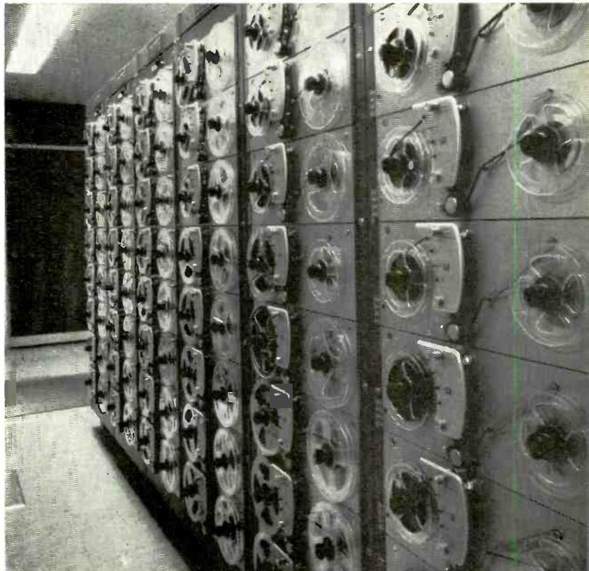
Bank of 188 audio recorders provide multitude of telephone-retrievable programs.
