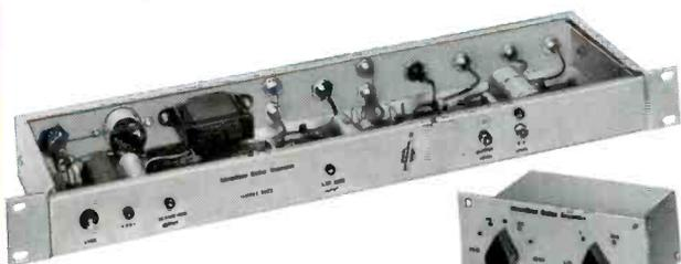
When used with any modern special effects equipment, this unit can create color titling and color matting from any black and white source. With the proper input signals a complete composite color signal is available for use with any modern production color switcher. Luminance levels are automatically set to approximate the values for 75% color bars. This is done by the hue selector switch. Saturation can be adjustable to suit desires. Has a one-year guarantee. \$675.00 FOB Nashville.
