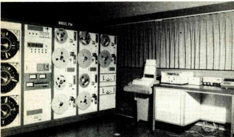
Sono-Mag DP-1 at WROC, Rochester, has five Scully tape decks (right-hand bays), three Carousels (at left end), with control equipment in center including full random access, and storage of 2048 events.
