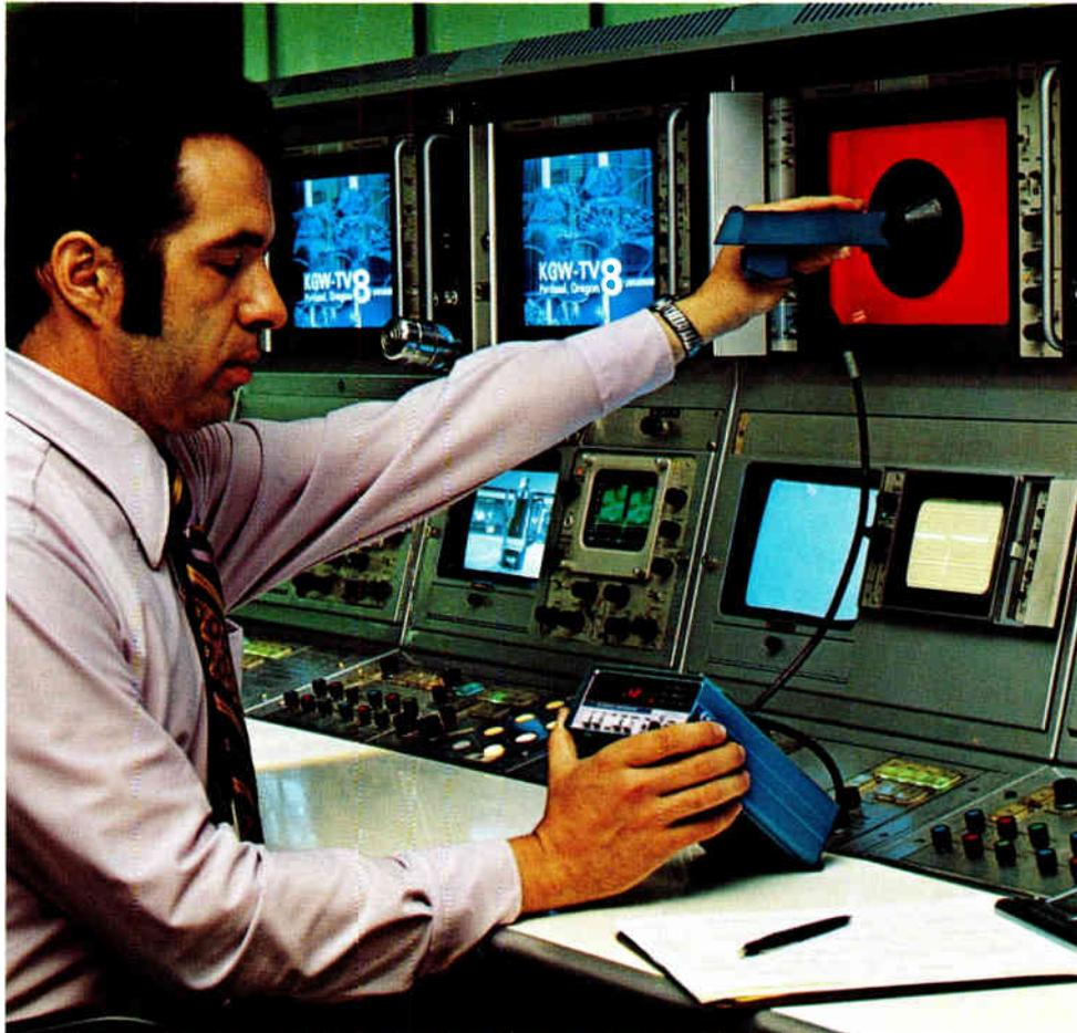
Improve color monitor performance with the TEKTRONIX J16-TV Photometer/Radiometer. Monitor screen color temperatures may be quickly and accurately adjusted or matched, even by unskilled personnel. No individual judgement is required as with visual comparison techniques.
