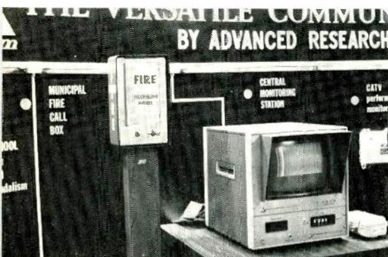
Fire and burglary alarm signals are traced to location by central CRT grid system in the Advanced Research two-way system. Circle 300.
