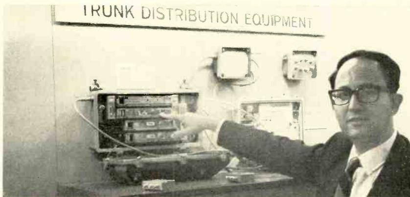
New Sylvania trunk amplifier has a sub-channel return amplifier for two-way. Circle 303.
