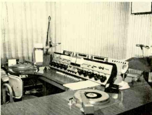
Diplomat console does not sit flat but is recessed on a slant into the cabinet.
