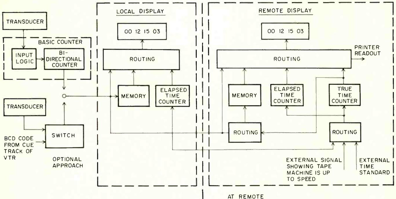
Figure 3. Block diagram of counting system.
