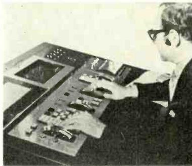
**Q-File**, uses computer techniques to allow one operator to activate many lighting cues through unlimited number of control channels. System controls up to four lighting cues simultaneously or in overlapping sequence, with manual override provision. Console surface under three square feet. **KLIEGL.** 276
