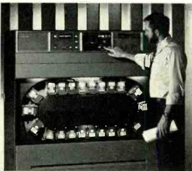
RCA's videotape cartridge system for automatic station breaks.
