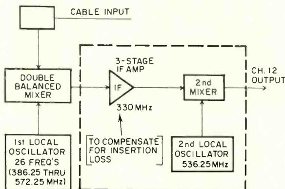
Block diagram of Gamut 26 converter which produces no interference signals. For more information, circle 300.
