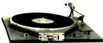
... is Spotmaster's new Studio Pro B, offering instant start and the tightest cue potential in the industry. Heavy duty hysteresis motor drives a 6½ lb. machined aluminum platter in a solid-cast aluminum chassis for inaudible rumble, lowest wow and flutter. Indicator lights tell speed (33 or 45) at a glance, and speeds can be changed with platter in motion. Detachable mounting plate (accepts any tonearm), integral 45 spindle and neutral cue position are other features ... all for just \$198.00.
