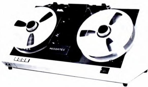
*Our transport uses a vacuum chamber for gentle tape handling, combined with vacuum grid cleaners to avoid scratching or cutting valuable tapes.*
