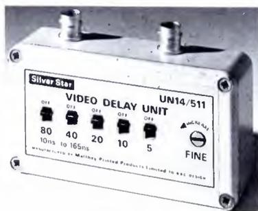
Infinitely variable range of 10-165 ns. in 5 ns. steps, selectable by switches, with fine trim of ± 4 ns. by screw adjustment. Cascade with fixed delay boxes of 50, 200, 500 and 1,000 ns. 75 Ω—fully-equalized—insertion loss .1 dB. In service at all three networks, numerous stations.
