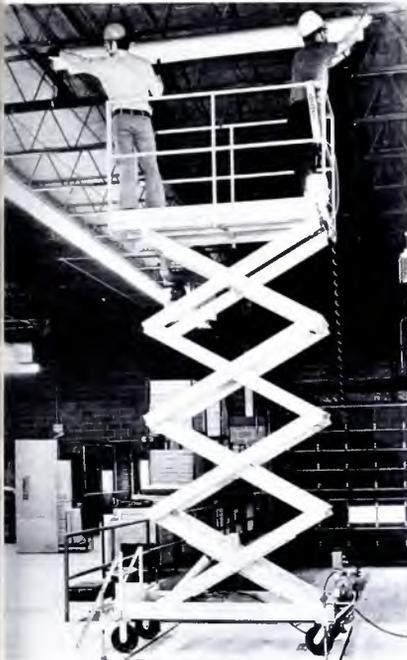
42-in. railing, operate on 115/1/60 power, and have duplex receptacle at the platform for power tools. ECONS MODEL ENGINEERING. **275**
