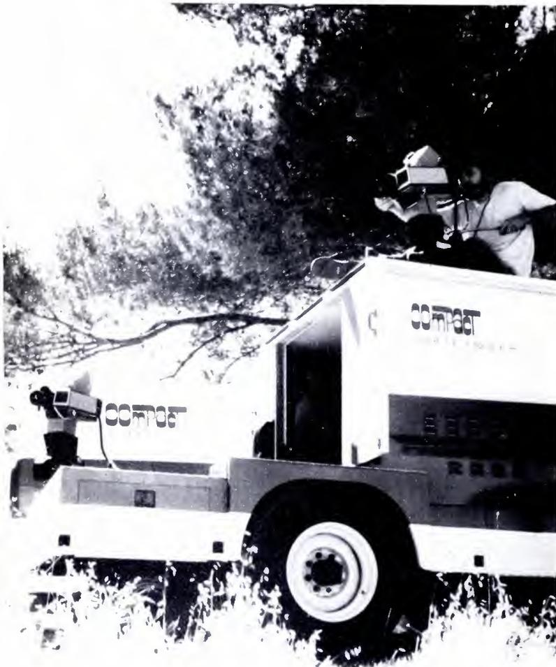
Camera-studio truck operating with camera on roof, another on open rear platform. Complete control studio is inside roofed part of truck. Power truck can be seen in background.
