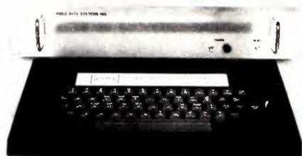
sync gives RS170 color or mono composite for display on standard TV set or video monitor. Other models accept 5-level baudot, 6-level stock ticker code, or other standard formats. VIDEO DATA SYSTEMS, INC. 298
