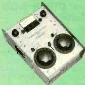
RG-1 RECEIVER/GENERATOR — Two-watt signal generator with a tracking detector. Built-in rechargeable battery power supply for full portability in making low power impedance measurements. For use with OIB-1 or other RF bridges.
