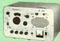
CPB-1 COMMON POINT IMPEDANCE BRIDGE — Monitors common point impedance continuously. Designed for permanent installation.
