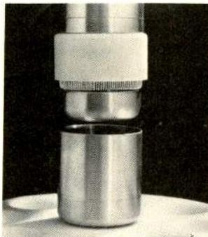
Unusual bullet connector from SWR catches wear particles in cup so they won't contaminate dielectric. Also instead of fingers that wear irreparably, contact action is confined to a replaceable wristband spring contained by Teflon sleeve. Photo shows lower half of transmission line before it is pushed upward to mate.
