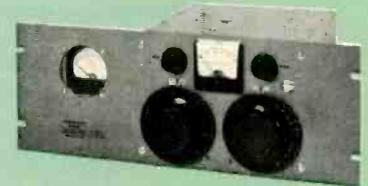
FSM-1 FIELD STRENGTH METER – Single frequency meter for simple, error-free, economical field strength measurements. Plug in modules for multi-frequency and harmonic measurements.
