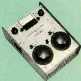
OIB-1 OPERATING IMPEDANCE BRIDGE – For antenna system measurements under transmitter power. May also be used as a conventional bridge.
