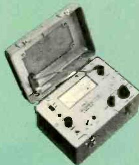
CPB-1 COMMON POINT IMPEDANCE BRIDGE – Monitors common point impedance continuously. Designed for permanent installation.
