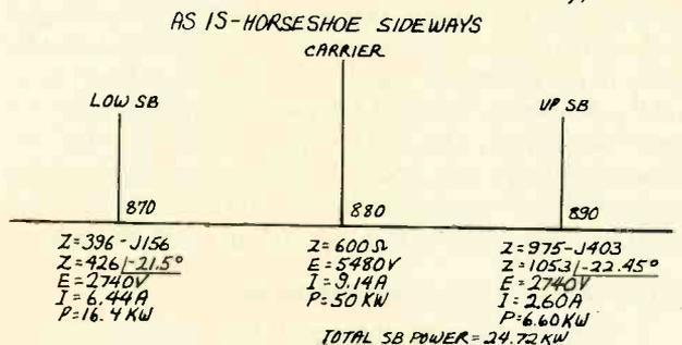
Fig. 2. Calculations show large variation in impedance between upper and lower sidebands of original Curve “A”. Fig. 3A (top right). Power and impedance distribution with 600 ohm load, showing even upper and lower sidebands. Fig. 3B (center right). Power and impedance with adjustment to Curve “B” shown on chart. Fig. 3C (bottom right). Calculations for Curve “C”, which was produced by a 45° delay network.
