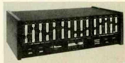
recorder, as well as open-reel, 1-inch VTR's. Dual joysticks control bidirectional variable speed tape motion of both playback and record VTR's. Options include switchable cross-pulse to the video monitor and programmable end insert timer. \$6,000. CONVERGENCE CORP. **305**
