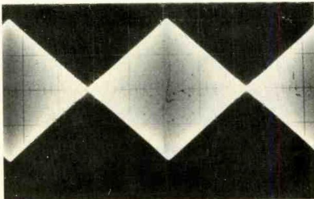
Fig. 8. A triangular waveform checks for non-linearity in the cross-over region, which can add significantly to distortion. In the example shown, the cross-over was found to be highly linear.
