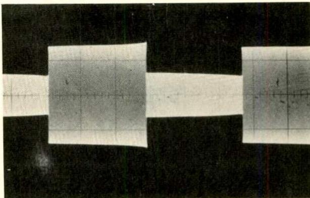
Fig. 6. Square wave at 20 Hz is check for low-frequency phase shift which might preclude clipping at low frequencies. In test illustrated, response is good down to dc.
