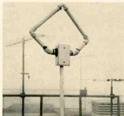
Completed antenna built out of PVC.
