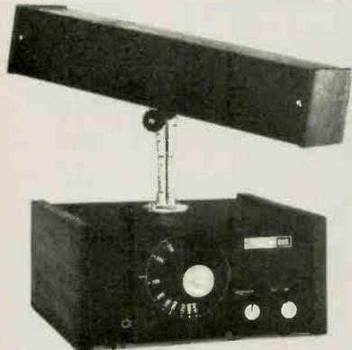
kHz whistle filter is built in. Frequency response is 15 Hz to 10,000 Hz. Sensitivity is  $3 \mu\text{V}$ . Companion (separate) ferrite antenna, the DA3, is shielded and directional with FET two-stage amplifier. It can be rotated and tilted to null out unwanted signals. McKAY DYMEK **300**
