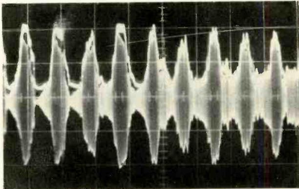
Fig. 7A. To check power supply bounce, and its limit on modulation, compare input and output waveforms of a complex audio signal. Test above shows considerable tilt and overshoot of 20-30%.
