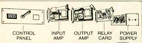
CONTROL PANEL    INPUT AMP    OUTPUT AMP    RELAY CARD    POWER SUPPLY
