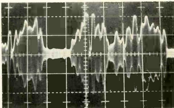
Fig. 7B. In this example of the input-output test, the pattern shows good tracking between the two waves, indicating a stable power supply.
