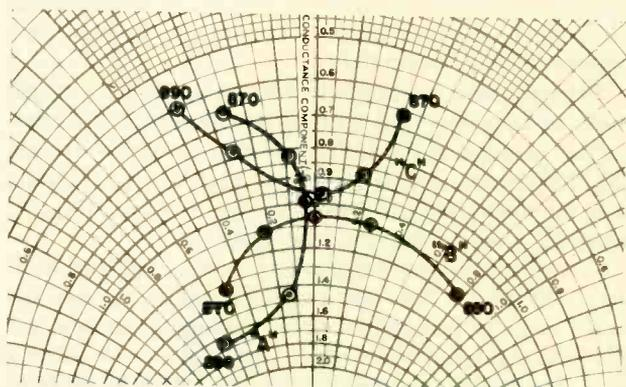
Fig. 1. Plots on Smith Chart show impedance-frequency curves of antenna. Curve A, the original, shows considerable variation at upper and lower sidebands. Curve B is a 45° advance; Curve C, which was chosen, a 45° delay,
