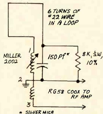
Schematic of loop monitoring antenna. A general discussion of the loop antenna can be found in the ARRL antenna handbook
