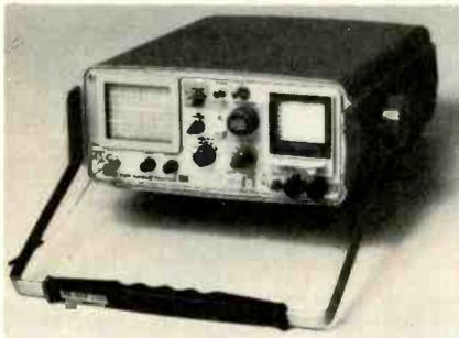
has maximum range of 2000 feet, and can identify impedance changes as small as 0.1 ohm. Model 1503 ranges to 50,000 feet, has 3-foot resolution, and is calibrated in return loss. TEKTRONIX **300**
