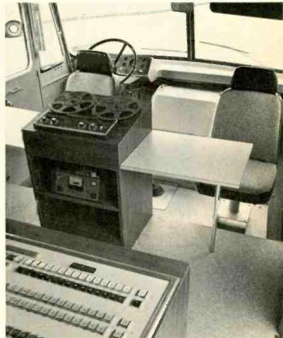
Interior shot of Mobile Television van used for special events broadcasting shows Tapecaster cart machine underneath a reel-to-reel machine. Van also carries three Ampex BC-230B color cameras.
