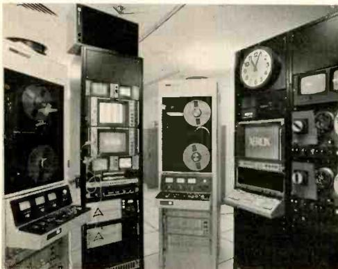
Fig. 6—Some of originating equipment in master control is Sony MV-10000 helical VTR, (left and center right), Datatron editor, TMI time base correctors, Tektronix monitoring and test units.
