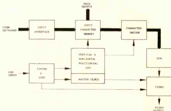
**Input Interface** Information from the keyboard enters at the Input Interface in digital or data form, such as USASCII data code, and is stored in a small buffer memory. Information can, of course, enter from sources other than the keyboard, such as magnetic tape or disc readers interfaced with the character generator.
