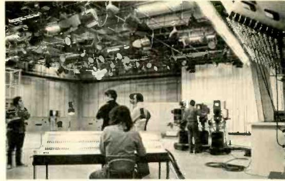
Interior of Studio A shows lighting control board in use. Three Ampex BC-230B color cameras are in use in the background. The control room is at the right behind glass.
