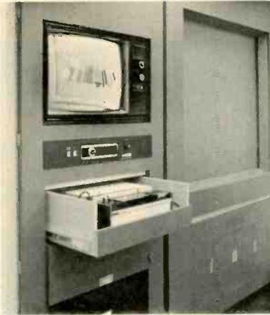
Fig. 3. (left) is close-up of AV/TV wall in classrooms. U-Matic player is in drawer, large rear-projection screen at right, communication panel in center.
