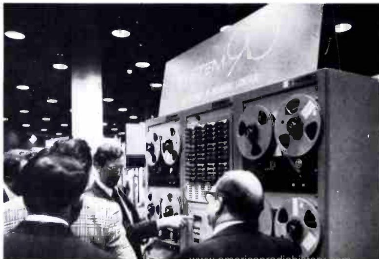
(Left) Harris System 90, here being pitched through its paces at NAB, Chicago, has micro-computer control, memory for 1,000 events, expandable with memory optics.
