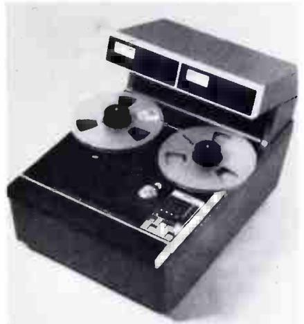
gramming. The ATR-100 features an exclusive tape handling system with fully servoed tape drive system. S/N ratio of better than 80 dB (full track at 30 ips) and an overall record and reproduce response of  $\pm 3/4$  dB, 100 Hz-15 kHz at 15 ips. Prices start at under \$5000. AMPEX CORP. **302**
