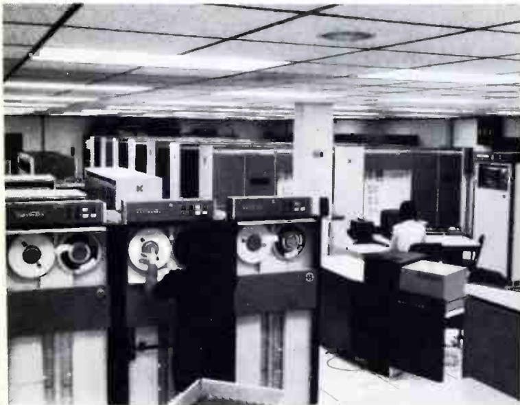
*In Memphis, BIAS uses its "super computer," Burroughs 6700, to handle most of the business computing for its clients. The machines are constantly on line to the station terminals (below).*
