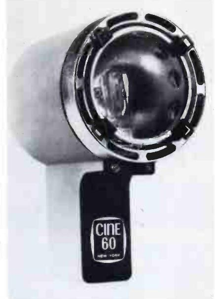
mounted, or on a light stand is available. "Jet-Lux" is a 115 V light which uses an 850W, 3400K lamp and will project a light beam of 150 ft at 10 ft, and has a built-in motor-driven cooling system, 7.5 ft power cable, 'thumb' switch to turn off lamp and other features. CINE 60, INC. 319
