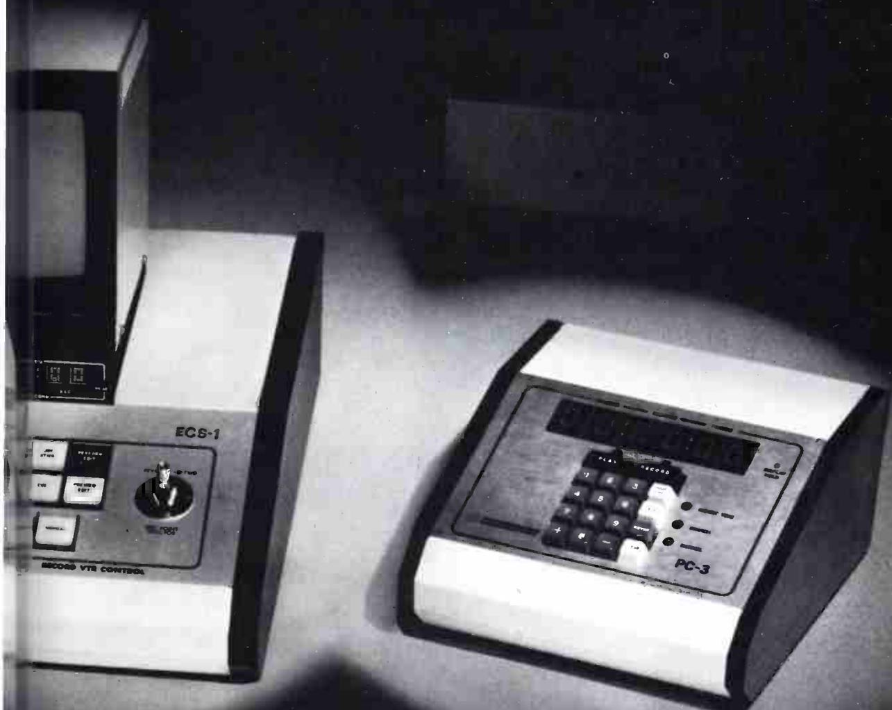
**TT-4 Digital LED Tape Timer** fits neatly under the monitor on a standard ECS-1. It counts control track pulses to tell you know where you're at and where you're going. It's what helical video tape editors have been looking for. The TT-4 counts up and down and can be reset to zero or set to any number. It even times assemble edits to show you accumulated program time. Buy it now or add it later.
