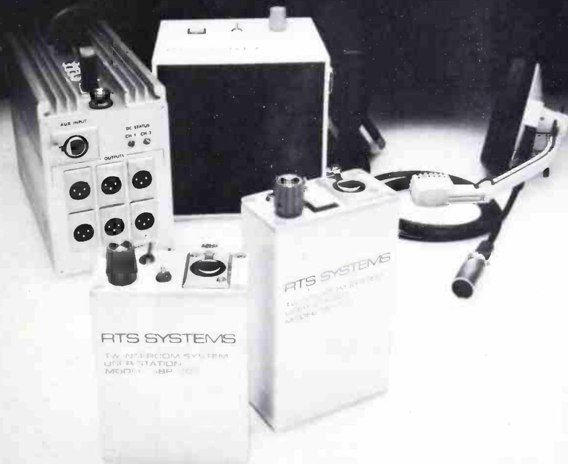
RTS SYSTEMS INTRODUCES THE MOST ADVANCED COMMUNICATIONS CONCEPT ON THE MARKET. THE TW INTERCOM SYSTEM: A refined, high-quality, and ultra-reliable intercom system for the demanding professional. Employing two wires for operation, up to fifty units may be connected in one without loading or serious performance degradation. Features include: mic level limiter, flashing signal light, auxiliary microphone input, adjustable side tone, and powerful two watt telephone amp.
