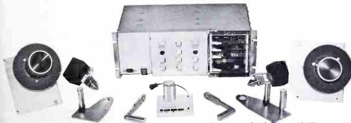
R-MOD (Reel-Servo Modification) makes your quad VTR handle tape with intelligence. R-MOD provides gentle tape handling, fast lock-up and fully automated operation including end-of-tape sensing. It provides all the desirable transport features
