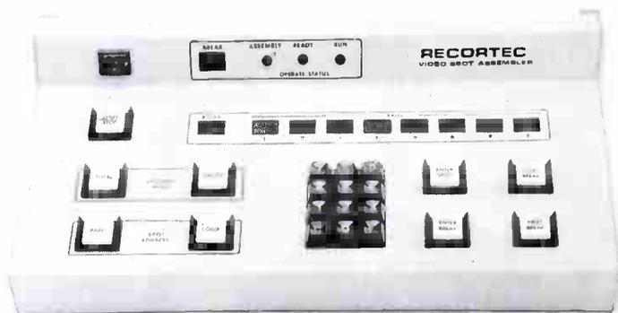
The Video Spot Assembler is a special purpose editing controller that makes spot reel assembly faster and easier. The VSA controls two existing VTRs to produce multi-break spot reels using less VTR and oper-
