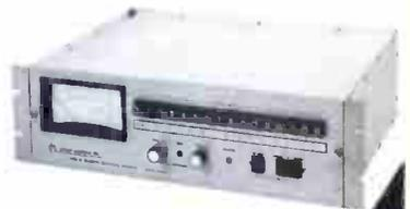
Fifteen telemetry and thirty command functions are provided by the **TRC-15A Remote Control System**. The **Model TRC-15AR**, when used in conjunction with a Moseley STL will provide totally wireless operation. The **Model TRC-15AW** is for use on leased telephone, or other wired circuits.
