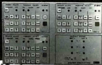
Microprocessor with 1536 bytes ROM (erasable), 512 bytes RAM, Provisions for 3 time base correctors, 3 VTR's, 3 Time code generators. Up to 4 control panels plus edit stations. Functional control. Priority assignment (on air, edit, microwave, record). Tally indicators (Assignments • Busy signal • Illegal path Lockout) Built in test routines. Multilevel machine control. Complete software reconfiguration. 20 x 16 + 28 x 1 + 2 (4 x 5) Matrices plus space for routing expansion.
