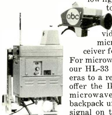
For microwave transmission from our HL-33 and HL-35 ENG cameras to a remote pickup point, we offer the Ikegami PF71 portable microwave relay system. This backpack unit transmits the video signal on the 13-GHz microwave band; audio and command signals on the 950-MHz uhf band. Maximum range is about 1800 feet with omni antenna, 3700 feet with 60-degree horn, two miles with a 20-degree horn.
