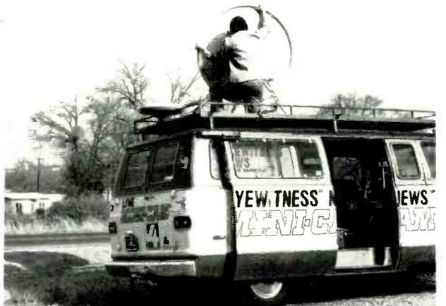
Raising the 2 GHz microwave transmitting dish and aligning it towards the receive site on Sandia Crest.
