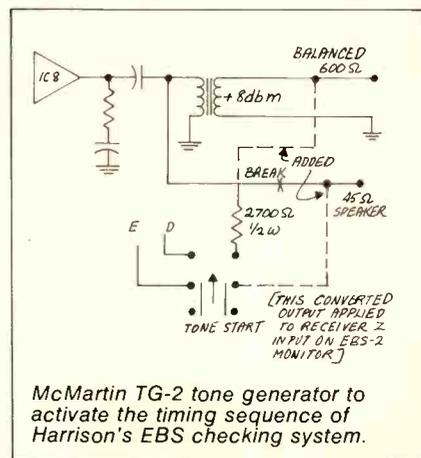
the contacts, as in the schematic. This output is applied to the Receiver 2 input on the McMartin EBS-2 monitor.
