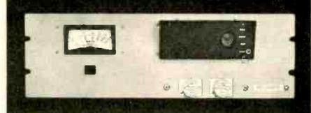
Offers Remote or On-Site Supervision of transmitters with 200 microsecond switching option to back-up plant. Visual and audible alarms are remote-resettable, if RF power loss or high VSWR conditions occur.
