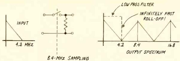
Fig. 9: Sampling at the Nyquist minimum of twice the highest signal frequency results in a spectrum which cannot be filtered correctly except by a filter with an infinitely fast roll-off—which is a physical impossibility.
