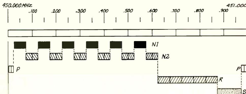
Chart shows new frequency assignments in 450-451 MHz band; those in 455-456 are the mirror image (order reversed), to double the bands shown, make 38 new frequency assignments. Service assignments are described in story; brand new are the P channels (telemetry) and S (composite stereo).
