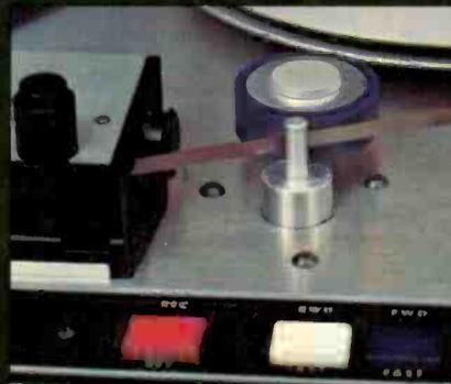
"This new high-friction polyurethane roller pulls the tape with less pressure. Less wow and flutter."
