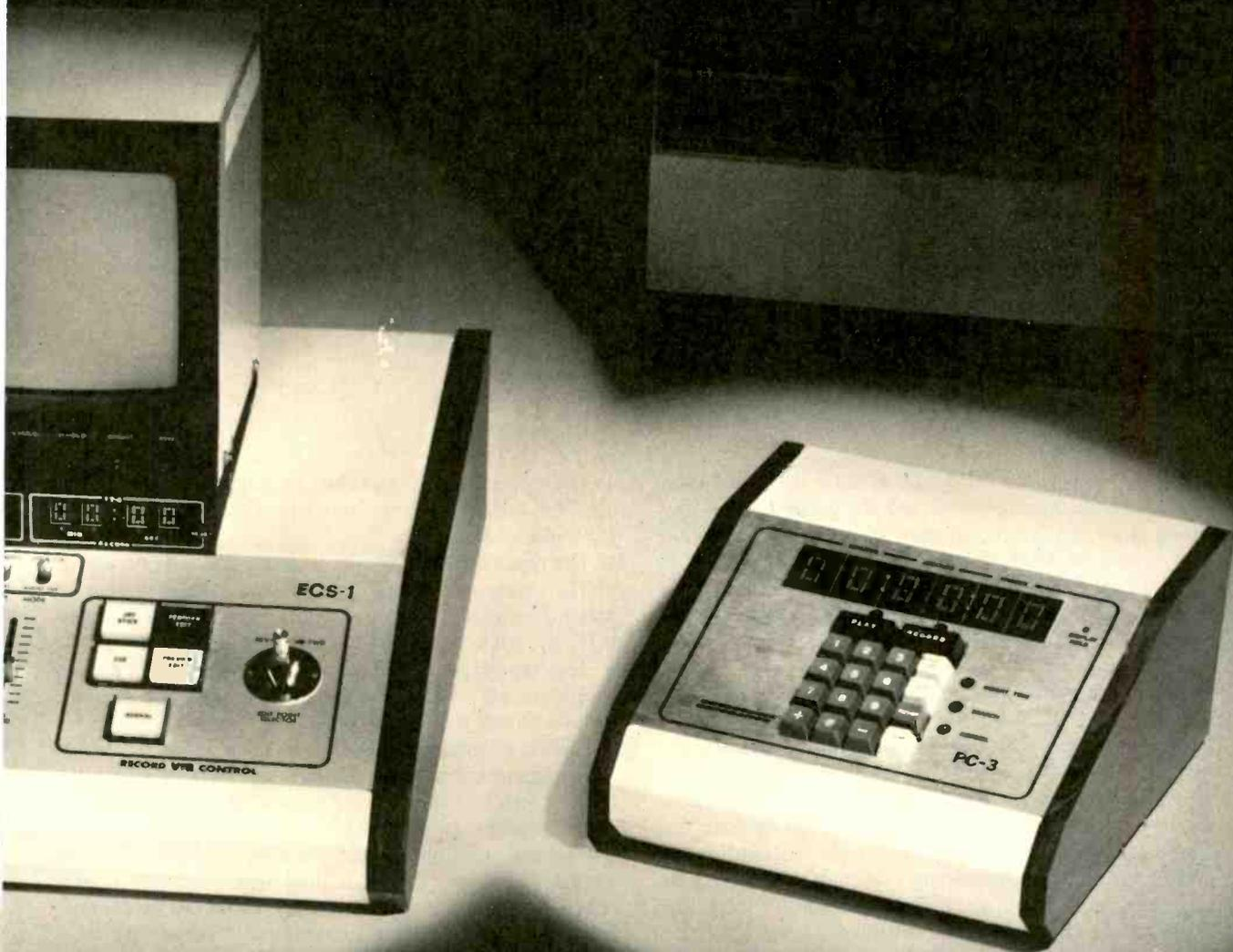
**TT-4 Digital LED Tape Timer** fits neatly under the monitor on a standard ECS-1. It counts control track pulses to let you know where you're at and where you're going. It's just what helical video tape editors have been looking for. The TT-4 counts up and down and can be reset to zero or preset to any number. It even times assemble edits to give you accumulated program time. Buy it now or add it later.
