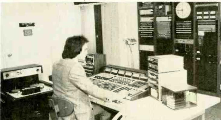
Master control for new Mutual system includes switching for routing incoming material to one of taping rooms or "on air," plus switching for outgoing feeds, ordinarily assigned by the computer. Console also has keyboard for entry of additional program events in computer memory; will have CRT read-out of program block (not installed at time of picture).
