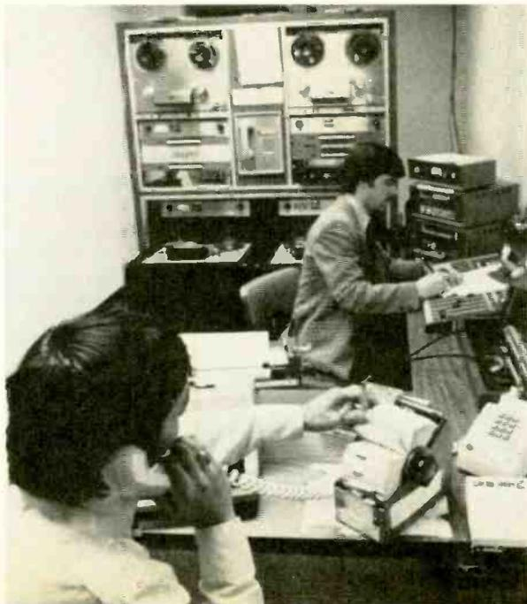
IGM Instacarts. The IGM system was modified by Mutual to meet the system requirements exactly. There is a series of Instacart trays in the master control room, each tray position with an identifying number marked alongside and entered in the switching. The computer "knows" all the numbers, rolls the cart at the tray position called for by number in the log sequence.
