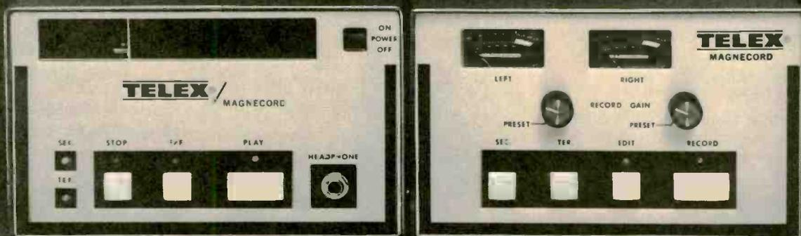
Telex/Magnecord broadcast cart machines run cool and steady. So cool no ventilation is required, so steady not even voltage or frequency fluctuations will alter their speed. Thanks to our dc servo flutter-filter drive.
