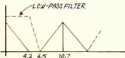
Fig. 10: Using a sample rate about 20% greater than the Nyquist minimum allows room for a reasonable roll-off rate for the filter. Sampling at 14.3 MHz yields even better filter management.
