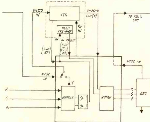
Tri Chroma black box takes RGB from camera and feeds it to VTR head in two bands: 7-10 MHz for Y and 2-3 MHz for R-Y and B-Y. Latter two are recorded separately in alternate fields.
