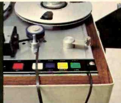
"Dumping tape in the edit mode is fast, easy, foolproof. Moving the tension arm down turns the take-up reel off. I can discard tape, listening as I go."
