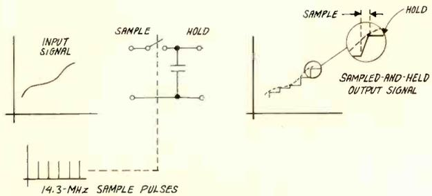
Fig. 7: A sample-and-hold sampling process. This is the process most commonly encountered in digital television systems. It unfortunately carries with it a frequency response problem.
