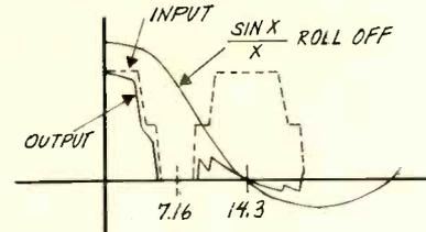
Fig. 8: The roll-off resulting from sample-and-hold type sampling. The original spectrum, shown dotted, has been shown with a step in it to aid in visualizing the roll-off action. This roll-off, which is 11% at subcarrier, must be compensated.
