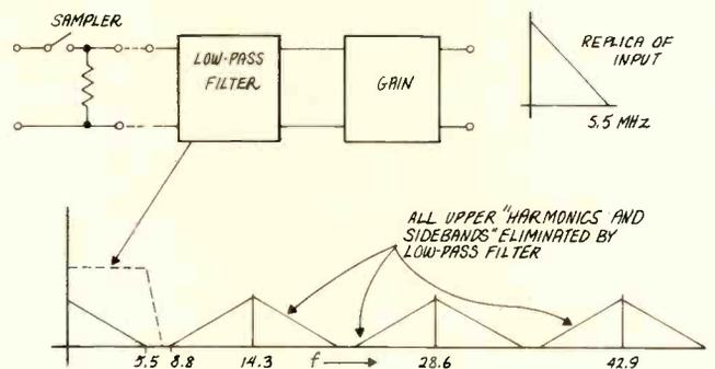
Fig. 3: To recover the original signal from the spectrum of Fig. 2, a low-pass filter is used to eliminate the undesired upper spectral components, and gain is inserted to restore the original amplitude.
