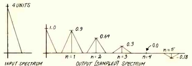
Fig. 5: The spectrum resulting from sampling with a 25%-duty-cycle pulse. Each successive harmonic group is reduced in amplitude by a factor derived from the mathematical gain factor  $\sin x/x$ , as explained in the text. Note that the baseband signal, though reduced 4-to-1 in amplitude, may still be recovered by simple low-pass filtering.
