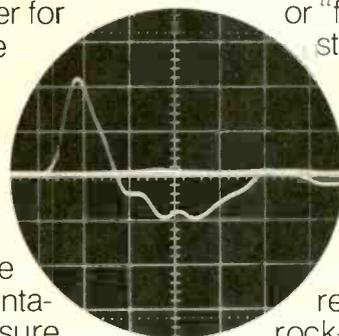
\*Outdoor test with Tektronix scope, set for 10V/division vertical, 01. μsec/div. horizontal. 22 cal. starter's pistol mounted 15 cm from MD 421 measured pressure of 111,000 dynes/cm<sup>2</sup> (175 dB SPL). Smooth, rounded scope trace indicates total lack of distortion.
