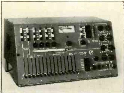
mastering, auditioning of mics and high level sources, variable equalization, reverb circuit, compression, cueing, testone, voice-over ducking, stage paging. Master control allows airing one program while recording another. ULTRA AUDIO PRODUCTS.
