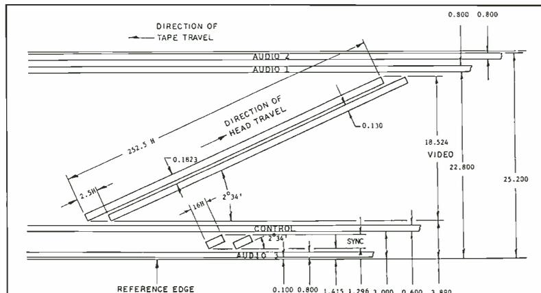
SMPTE Type C 1-in. helical video recording format. Proposed record locations and nominal dimensions.
