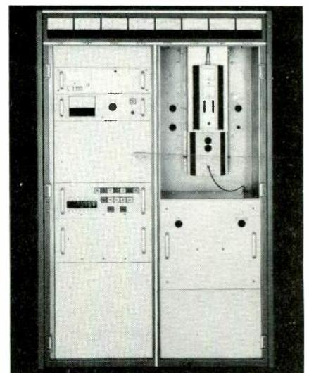
use quarter-wave reentrant cavities. Models TX-10, TX-100 and TX-1000 have low-level IF modulation, CMOS logic circuitry for both local and full
