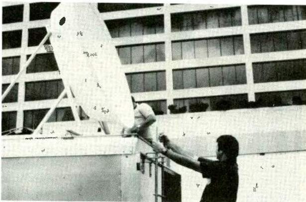
Program produced on location is beamed by satellite to other hospitals. Transmitter antenna (12 GHz) is beamed at experimental CTS satellite.
