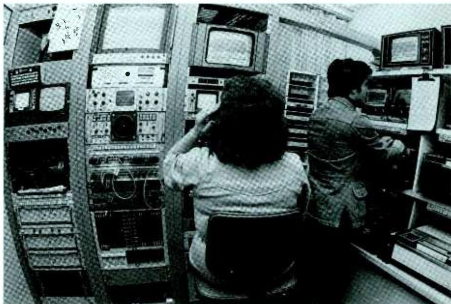
Eye Control: the heart of the ENG newsroom. Microwave controls are on left, patching and test gear in center rack. Two Microtime 2020s, one with Image Plus, are in righthand rack.
