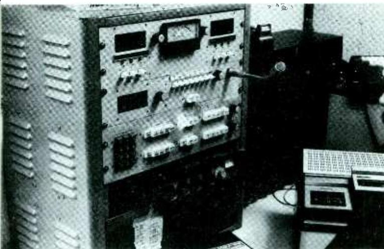
*Console in ENG decision room allows communications with all areas of WFAA operation through intercom system. Any in-house source can be routed to station's editors.*
