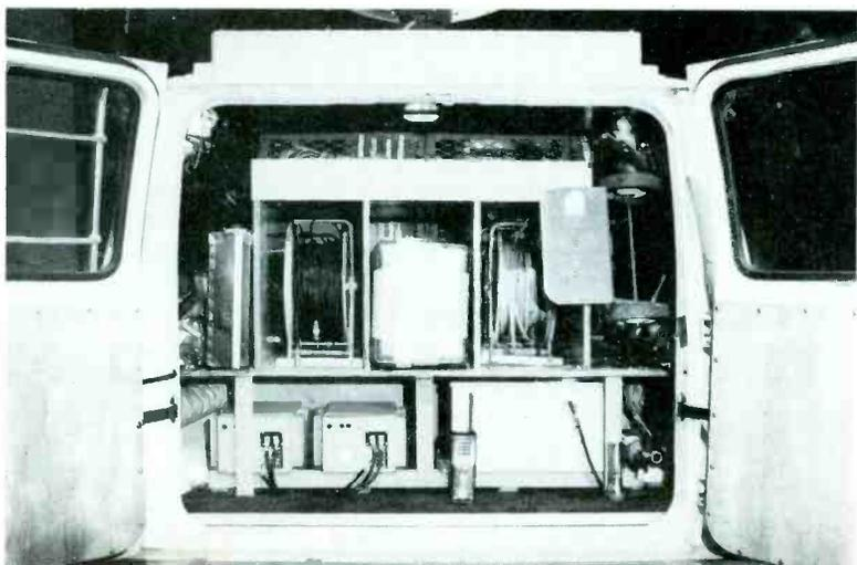
Easy access is provided to field equipment through rear doors. Van was designed at the station.
