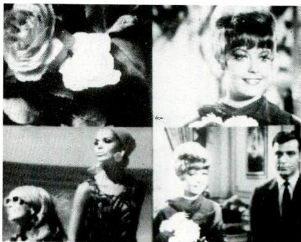
A "quad split" picture display processed in the BCN Digital Store from a single input. Alternatively, each of the quadrants can be filled with a different image, one of them a "moving picture."
