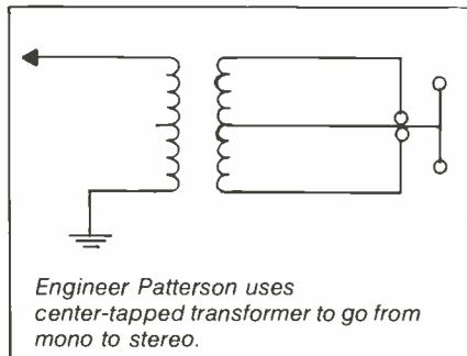
Engineer Patterson uses center-tapped transformer to go from mono to stereo.
