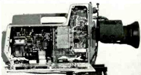
Merely opening the sideplates of the MNC-71CP permits checking all internal circuits without using a module extender.
