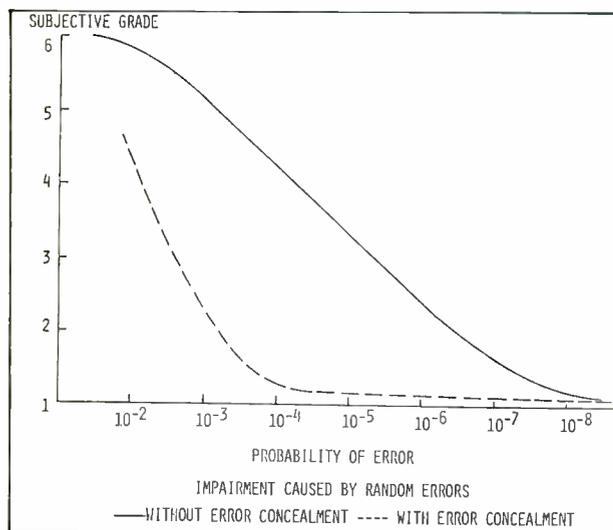
Fig. 6. Example of measured results for bit error rate sensitivity with PCM coding.
