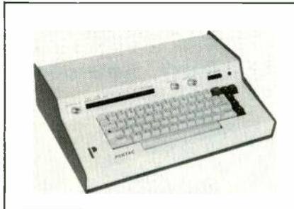
control for editing, adjustable-speed horizontal crawl, 16-digit line, and 8-line page. The memory holds 4 pages. It is microprocessor controlled, and automatically "fences" a \* symbol and resets to the beginning of the message for continuous loop operation. Brightness is controllable, and display size is selectable from 14 to 28 lines digit height. Numerous options are available for additional operating features. \$1,195.00. PORTAC. (Exclusive marketing, VIDEO COMPONENTS, INC.)
