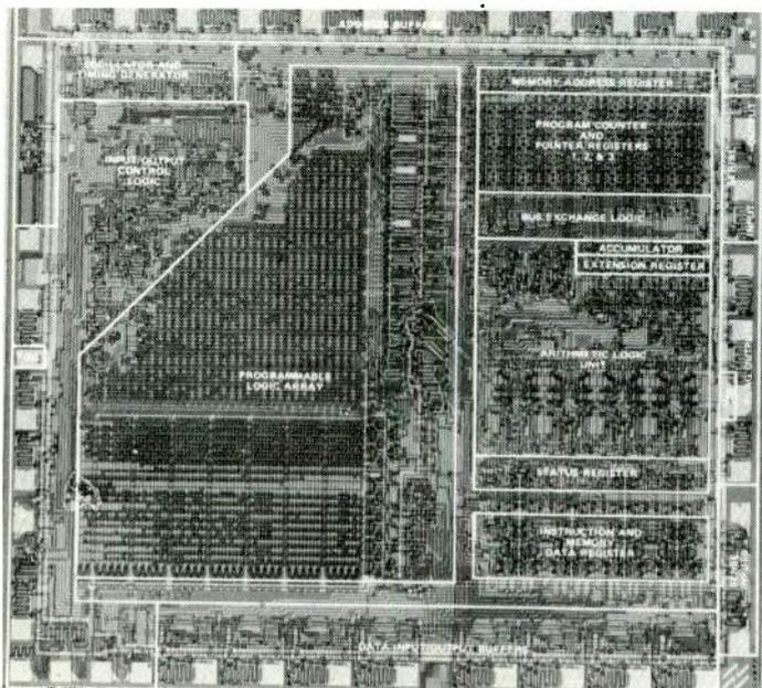
A typical microprocessor. Devices such as these will be taking on increasing importance in broadcast engineering.
