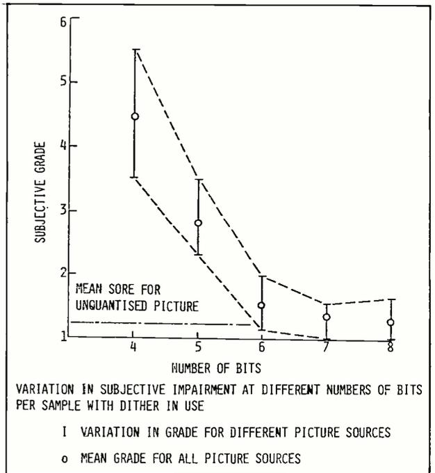
Example of measured results for PCM coding.
