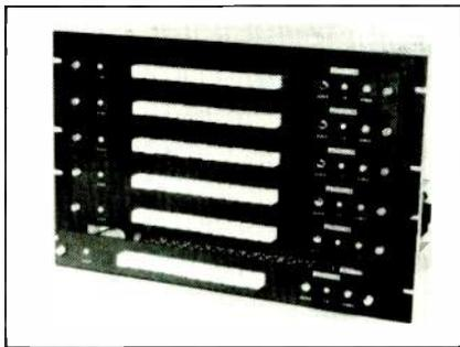
six of its modular units. Each module has both video and audio switching and a self-contained power supply. System can handle up to 12x12 without serious signal degradation. DYNASCIENCES.
