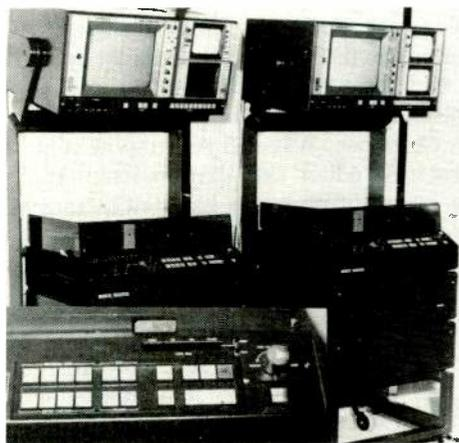
*Fig. 1. Bosch-Fernseh EES-9 Editing System provides control of Search, Assemble and Video/Audio 1/Audio 2/Audio 3 editing functions for two units from either console. Controller reads either SMPTE time code or longitudinal tape time at flip of internal switch. Insert shows right hand control panel details.*
