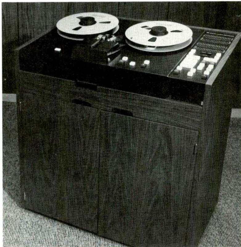
*Digital tape recorder developed by the 3M Company handles in much the same way as standard professional recorders. All operating controls are on panel at right, which lifts out of cabinet and moves up to 20 feet away for remoting.*
