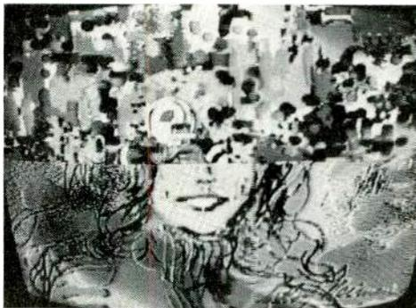
A Nieman rendering of CBS Sports commentator, Phyllis George is being replaced by another Neimen picture from the AVA frame buffer, line by line. An alternative display method is to read-out sequentially, which would allow the viewer to see the artwork recreated in the same sequence in which it was drawn.
