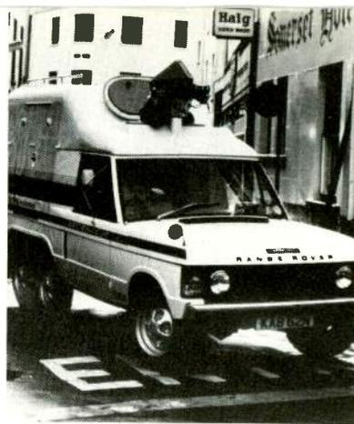
RCA constructed Range Rover van uses roof turret for camera mount.
