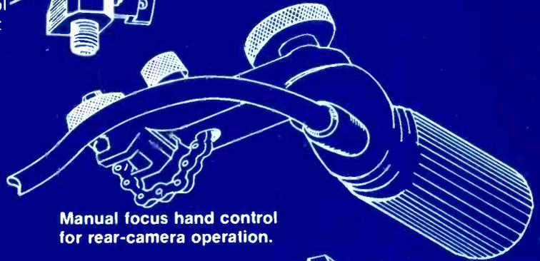
Manual focus hand control for rear-camera operation.
