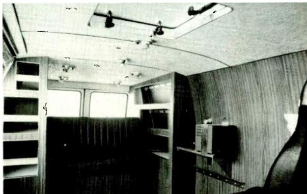
interior of WGBH's field production van by Wolf Coach. This configuration reflects the intention of WGBH to use the van for remote recording. Because the van is used for remote production and not news, more room is provided for personnel.
