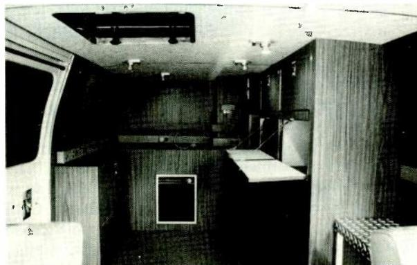
Another configuration for the interior reflects the intention to use the van as a production center. Wiremold is installed around the interior to provide a maximum number of power outlets since actual layout of equipment may change from day to day.
