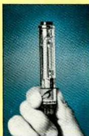
**Type XQ1427:** Offers significantly higher resolution than earlier versions; modulation depth is 60% typical at 320 TV lines giving sharper, clearer pictures and allowing operation at lower light levels. New gun design and 1500-line mesh construction result in improved registration and geometry, reduction of flare by a factor of 3 and reduced beam landing error.
