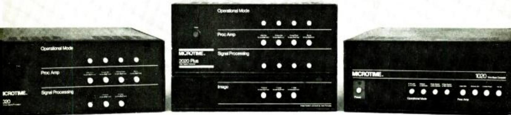
Solve those all important wide blanking problems with MICROTIME's Super Wide Window available on all 2020 Plus, 2020 ESP and 1020 Time Base Correctors. The exclusive Super Wide Window option offers a 24 line correction range to guarantee correct vertical blanking, by providing TBC output blanking per FCC specifications.
