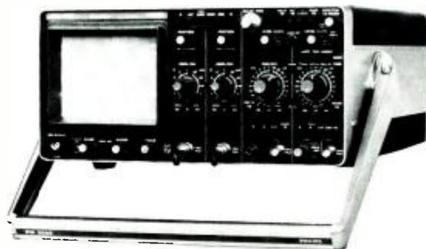
100MHz scopes with dual trace capabilities, such as this Philips Model PM3262, will be making their appearance at broadcast stations as more of the broadcast plant becomes digital. Scopes of this speed manufactured by Tektronix, Hewlett-Packard, and others have found general applications in manufacturing and computer fields
