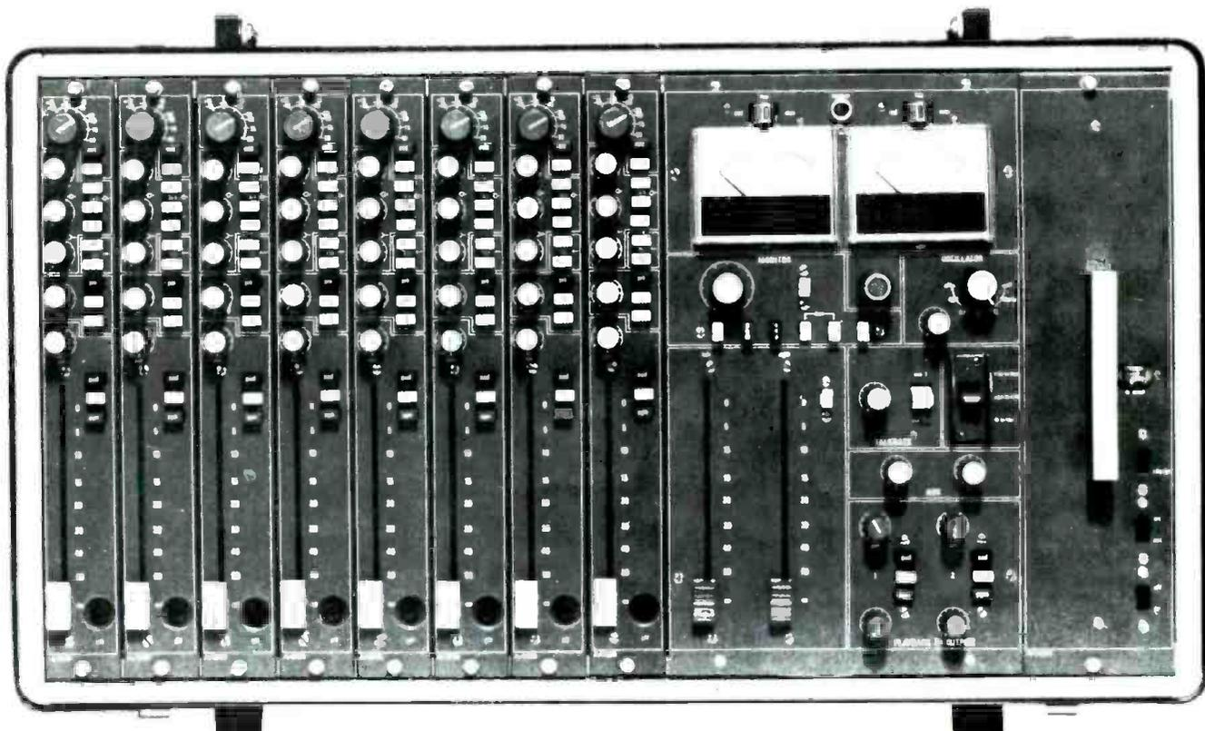
The all new Neve Model 5422 Suitcase Sound Mixer is designed to provide the broadcast, sound recording and film industries with a high quality portable mixer. It features 8 inputs with equalization, 2 main outputs, 2 auxiliary outputs and a lot of other facilities. External mains supply and rechargeable battery pack are available.
