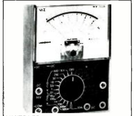
color coded scales. It measures dc voltage as low as one mV and up to 1,000 V in eight ranges; dc current from .1  $\mu$ A to 10A in seven ranges; resistance from .25 to 20 megohms in four ranges; and decibels from -20 to +36 dB. VIZ MFG CO
