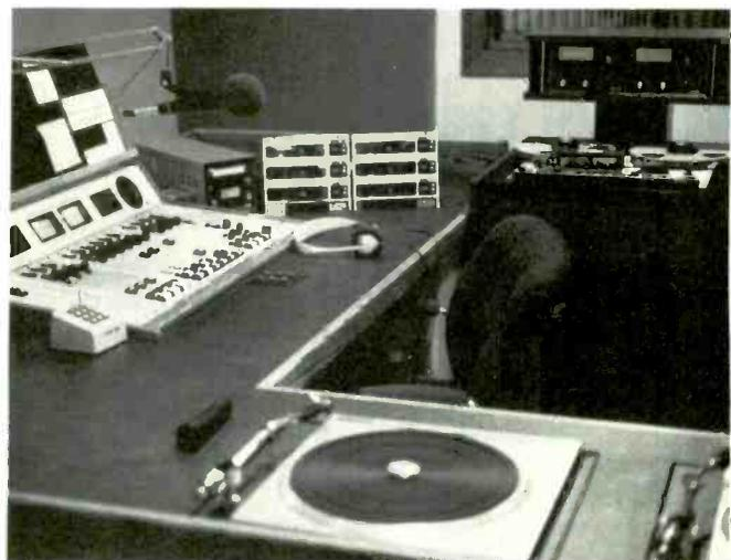
*KAAM's master control room. ITC cart units, Scully stereo decks and electronic turntables are mixed through a BMX-12. Two carbon-copy control rooms guarantee against down time*
