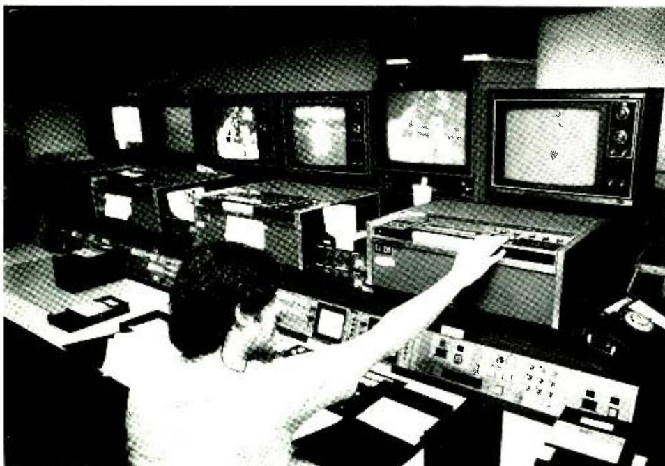
*KNBC's record/playback room contains four BVE-200s. Three decks, routed through Microtime 2020+ TBCs and the ADC switcher, are used to originate videocassette playbacks for local news programs. Fourth deck, connected to routing switcher outputs, records incoming feeds from the six microwave links, telco lines, East and West Coast NBC network feeds, etc. Almost all taped material used on local news programs is recorded, edited, and played back on 3/4-inch videocassettes*
