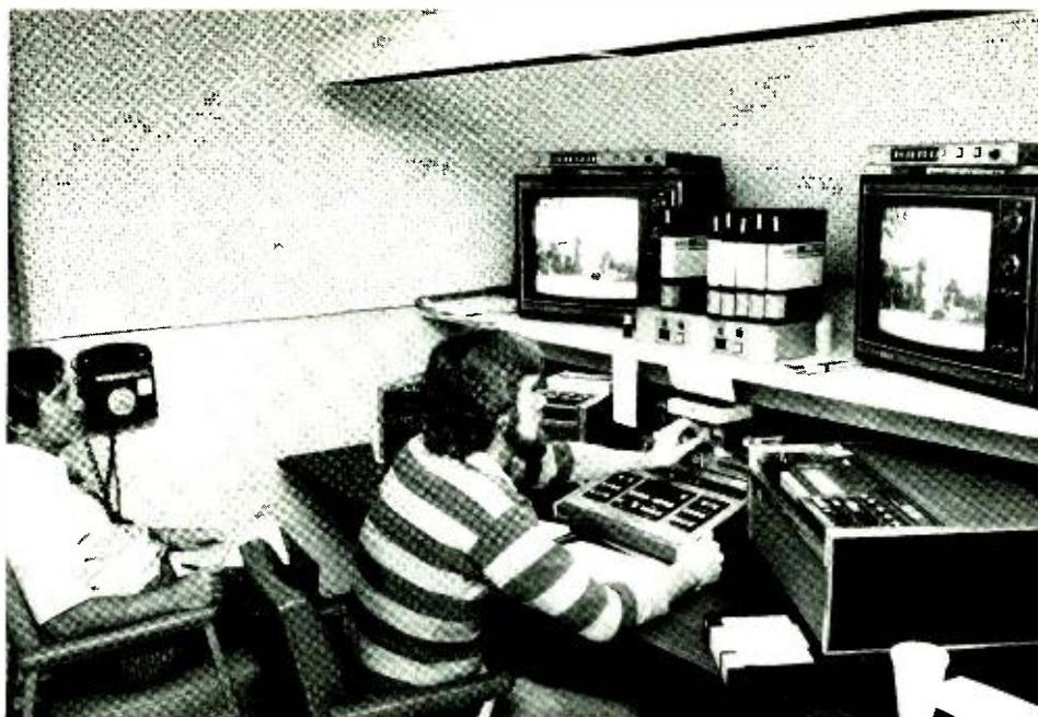
6:00 – 7:00 p.m., a half-hour from 11:00 – 11:30 p.m., and 10 minutes at 1:00 a.m. Four Convergence editors — two ECS-1s interfaced with Sony VO-2850s and two ECS-1Bs interfaced with Sony BVU-200s — handle the editing workload. One of the ECS-1B systems is assigned to the production area, but is frequently called into use for news starting around 4:00 in the afternoon when most of the tapes have arrived at the station. Each of the four editing systems gets at least five hours' use a day.
