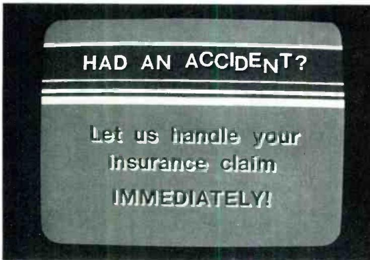
Typical local commercial message produced by Compositor I. Note the drop-shadow effect, variable baseline in the word "accident" and individual colorization of extremely small areas
