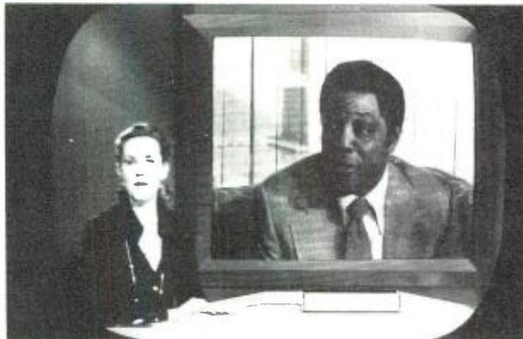
*The inset of Willie Mays is not keyed in but rather compressed and positioned to equate to the chroma key area. When the scene goes to the tape, the inset picture is automatically expanded and centered by the DVP as a box wipe*
