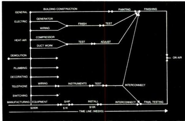
"PERT chart" is example of planning technique that allows different parts of complex job to be timed so that parts can be finished to allow others to start. Technique also allows detailed cost control and accurate scheduling of the job finish
