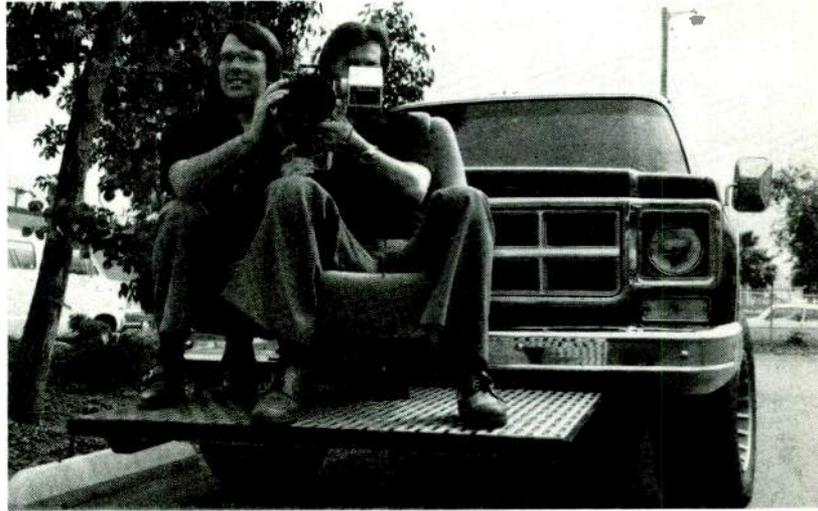
*The Centro-designed EFP vehicle for Sunset Productions incorporates a detachable front-mounting camera platform. The vehicle's customized suspension system permits completely steady operation during running shots*
