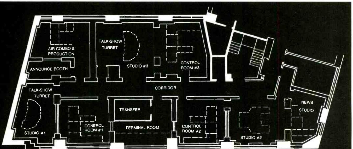
Floor plan shows how studios were laid out for mutual effectiveness. Studio 2, also in photo above, has adjoining room for control engineer when on-air talent requires one. Announce booth next to production room allows voice track to be added to commercials or other material
