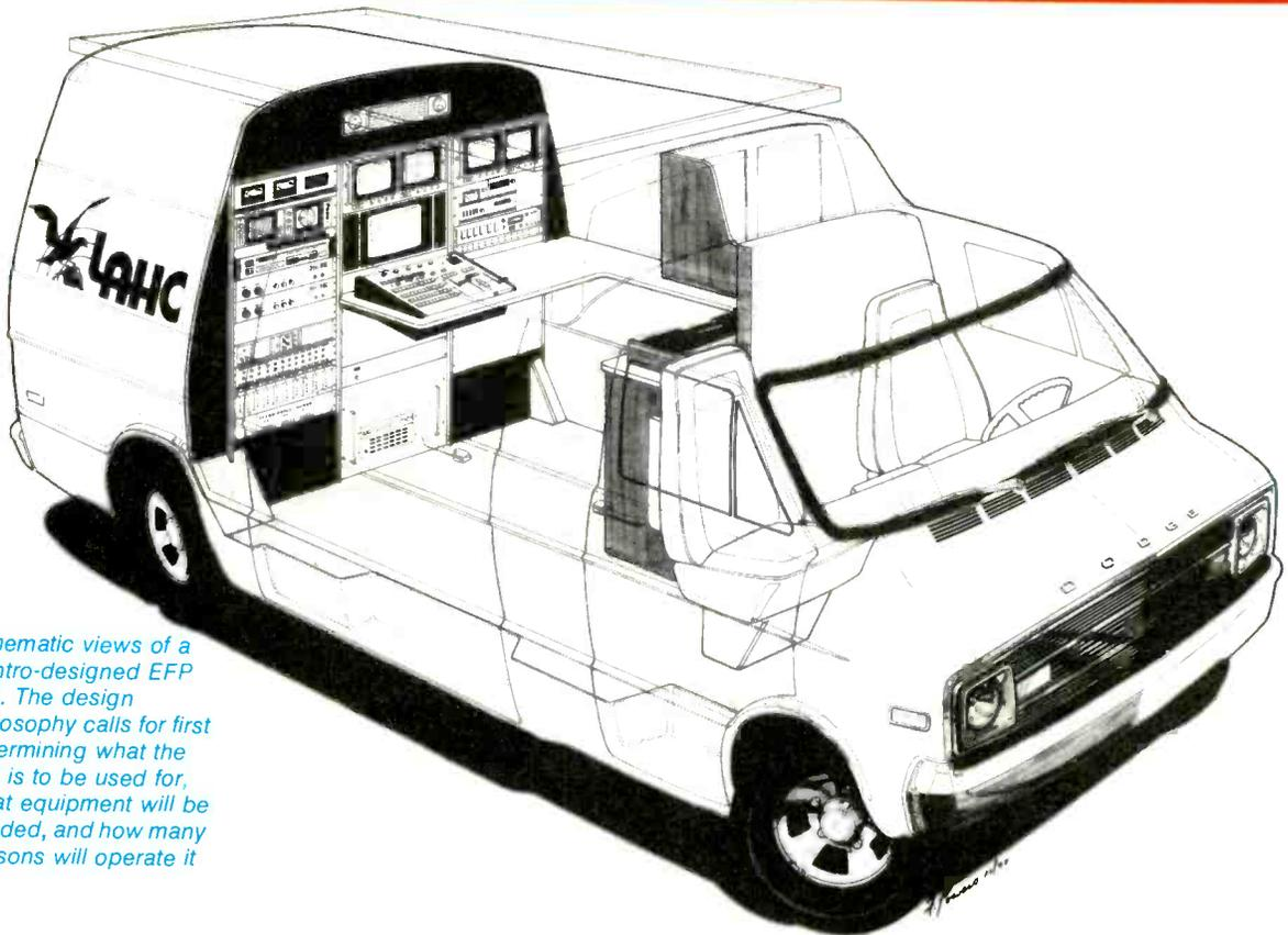
*Schematic views of a Centro-designed EFP van. The design philosophy calls for first determining what the van is to be used for, what equipment will be needed, and how many persons will operate it*
