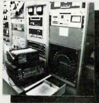
The Amber 4400A offers versatility and quality. Its features include sine, function, sweep, tone burst and noise generator; autoranging digital dBm meter and frequency counter; multinode filter; spectrum analyzer; frequency response and phase response plotter. High performance: low distortion and high output together with high measurement sensitivity and resolution.
