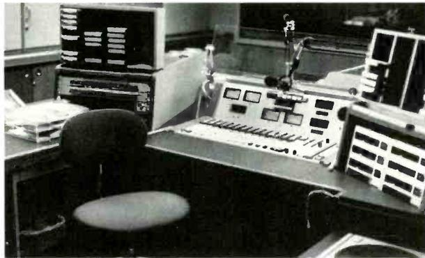
On-air position for talk personalities who use an engineer for control (studio 2 on diagram) can also be operated combo. Control, through window at rear, can go on the air independently. Rows of buttons (left) are for cross-bar switching (see story)
