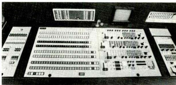
Control room console at Outlet Broadcasting's WJAR-TV. Vital 1600 switcher is the meta-controller
