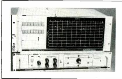
plays, individual gain-adjustable input amplifiers, programmable output cards for stereo and/or mono feeds, dual instantaneous switchover power supply, and balanced in and out. Response is  $\pm 0.5$  dB, 20 Hz to 20 kHz; distortion is 0.3 percent maximum; gain is variable (each input) +15 dB; S/N is -75 dB below +8 dBm out. From \$1099. RAMKO RESEARCH.
