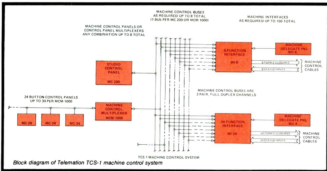
wind, fast forward, stop, in and out edit points, etc. — can be controlled through the central system. In addition, an override model allows the operator to put the machines into sync and then offset one machine relative to the others to achieve true audio sync. GPIB relay closures are provided for starting up special effects and other devices. Further, the system can be interlocked to the time code output from any VTR in the plant with the audio decks set to chase the VTR's time code.
