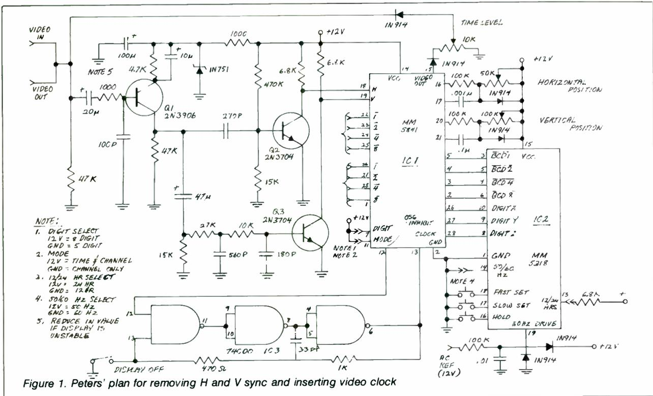
Figure 1. Peters' plan for removing H and V sync and inserting video clock
