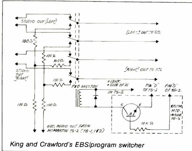
output is provided by the generator (such as the McMartin TG-2). One solution is to simply go through a pot on the board, but that is often impractical and demands that the operator remember to turn the pot up.
