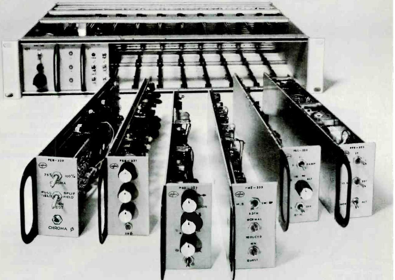
This totally integrated modular video test set is designed for the discriminating professional. The Lenco 300 System lets you specify video test signals to meet your system requirements, not the manufacturer's.
