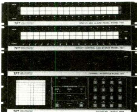
Time and Frequency remote control unit (above) and Moseley Associates' MRC-1, below. These two units are examples of the new generation of "smart" systems that take advantage of microprocessors in order to enhance the effectiveness of the human operator
