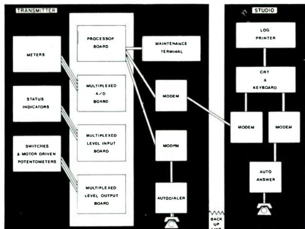
Block diagram of Telesis transmitter monitoring system. Sixty-four control channels operate external functions
