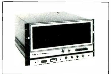
is the claimed result. A TBC is built into all units; front panel selectable field or frame picture freeze is standard. In addition, a DMA (direct memory access) I/O interface opens up such applications as digital still store and image processing. Digital noise reduction is available as a plug-in option. \$24,990. CONSOLIDATED VIDEO SYSTEMS.
