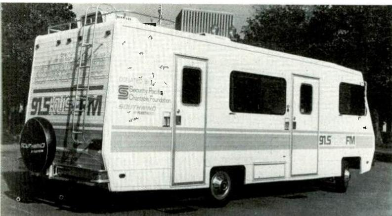
*Outside of mobile studio built at KUSC-FM, University of Southern California, for production of stereo tapes of concerts, and also for feeding the concerts live to the National Public Radio satellite net. The van has top-grade control, monitoring, and recording units, including Audiotronics multi-channel console, Studer tape machines. NPR uplink transmitter will be reached with a microwave system*
