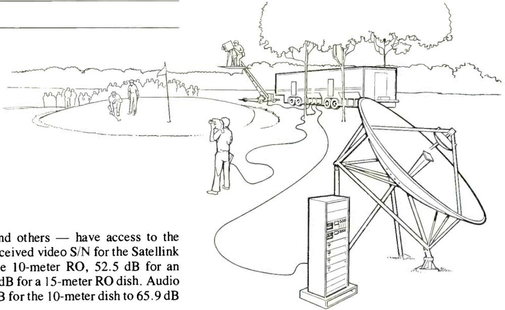
Storer Broadcasting, and others — have access to the larger earth stations. Received video S/N for the Satellink system is 52 dB for the 10-meter RO, 52.5 dB for an 11-meter RO, and 55.2 dB for a 15-meter RO dish. Audio S/N ranges from 62.6 dB for the 10-meter dish to 65.9 dB for the 15-meter dish.
