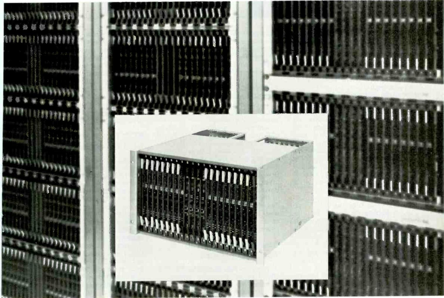
The Grass Valley Group proudly presents the 440 Series, an all new routing switcher of uncompromising design and performance. Its virtually transparent signal paths, fail safe reliability, and field expansion capability make it the routing switcher for the 1980s.
