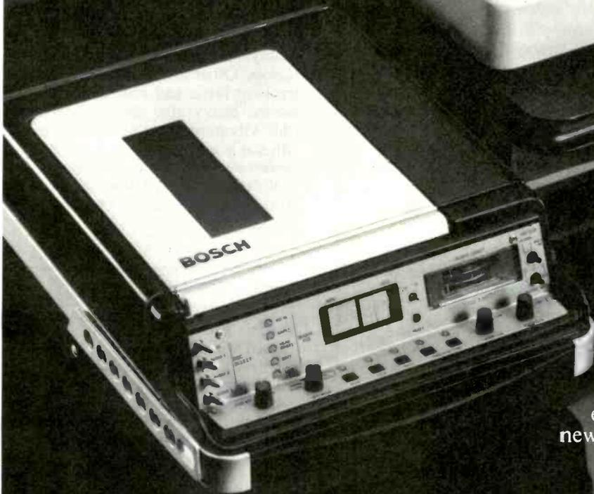
The first portable studio quality recording system with reels and cassettes 1 inch type B format according to SMPTE/EBU operating in all TV standards throughout the world.
