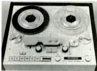
Studer A80 shows exceptionally "clean" top-panel layout, straight-line threading
