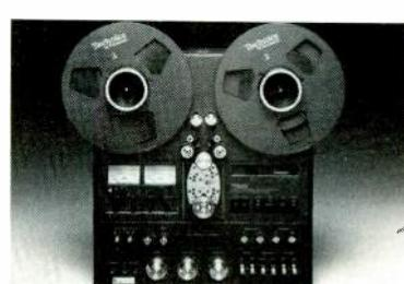
Technics (Panasonic) RS1520 has isolated-loop tape drive, crystal-locked capstan speed
