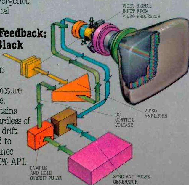
Conrac's unique system uses a keyed back porch video amplifier and beam current sensing that occurs during the vertical interval.
